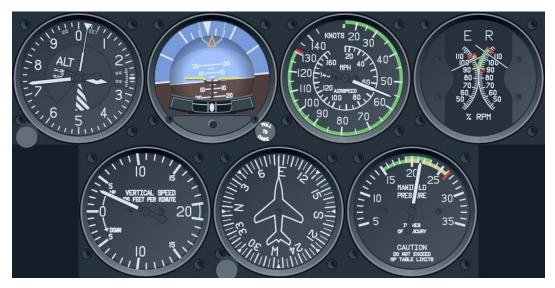
Figure 12 Robinson R44 instrument panel to be used in the Helicopter Pilot Station. The instruments include an Attitude Director Indicator and altitude and speed dials.
