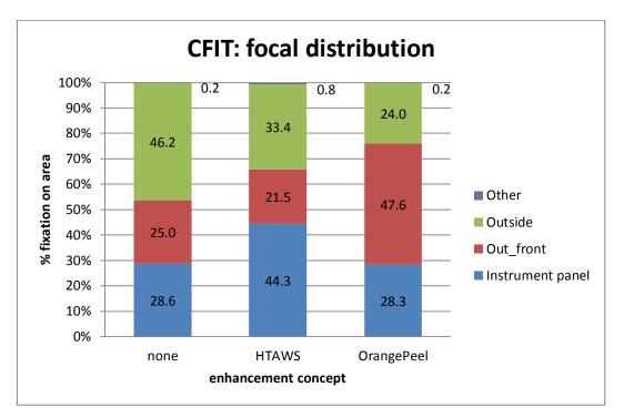
Figure 39 Focal distribution in the CFIT scenario for the enhancement concepts
