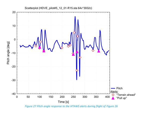
In most cases the pitch angle increased by from  $5^{\circ}$  to  $20^{\circ}$  or more due to pilot's action upon the alerts.
