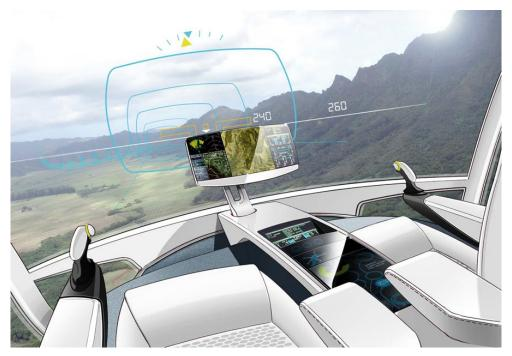
*Figure 5 Future rotorcraft cockpit with Malcolm Horizon (Courtesy Eurocopter)*
