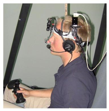
Figure 9 Eye tracker mounted on head of test subject
