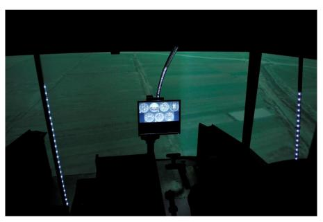
Figure 14 LED concept of three strips/poles in the cockpit
