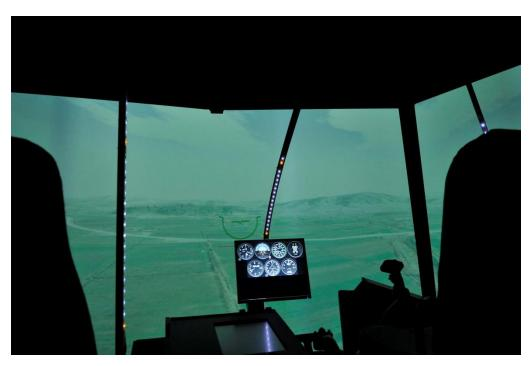
Figure 15 LED concept with amber-colored upward-traveling lights
