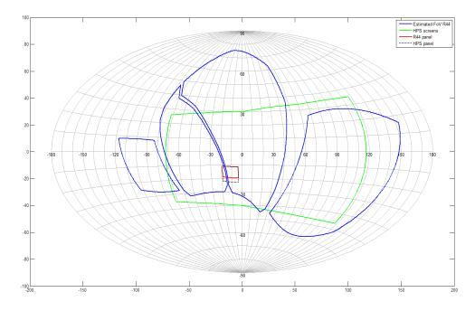
Figure 11 Optical field-of-view from the pilot's eye reference point in the HPS, with the new 19" instrument panel, relative to the R44 helicopter; HPS rotated 21.75<sup>o</sup> left relative to centerline
