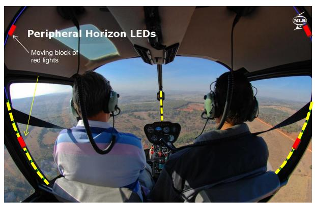
Figure 8 Lights (LEDs) mounted in the peripheral view of the pilot
