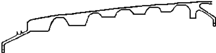
4.a - Ring Disk Drum Rotor Cross Section
