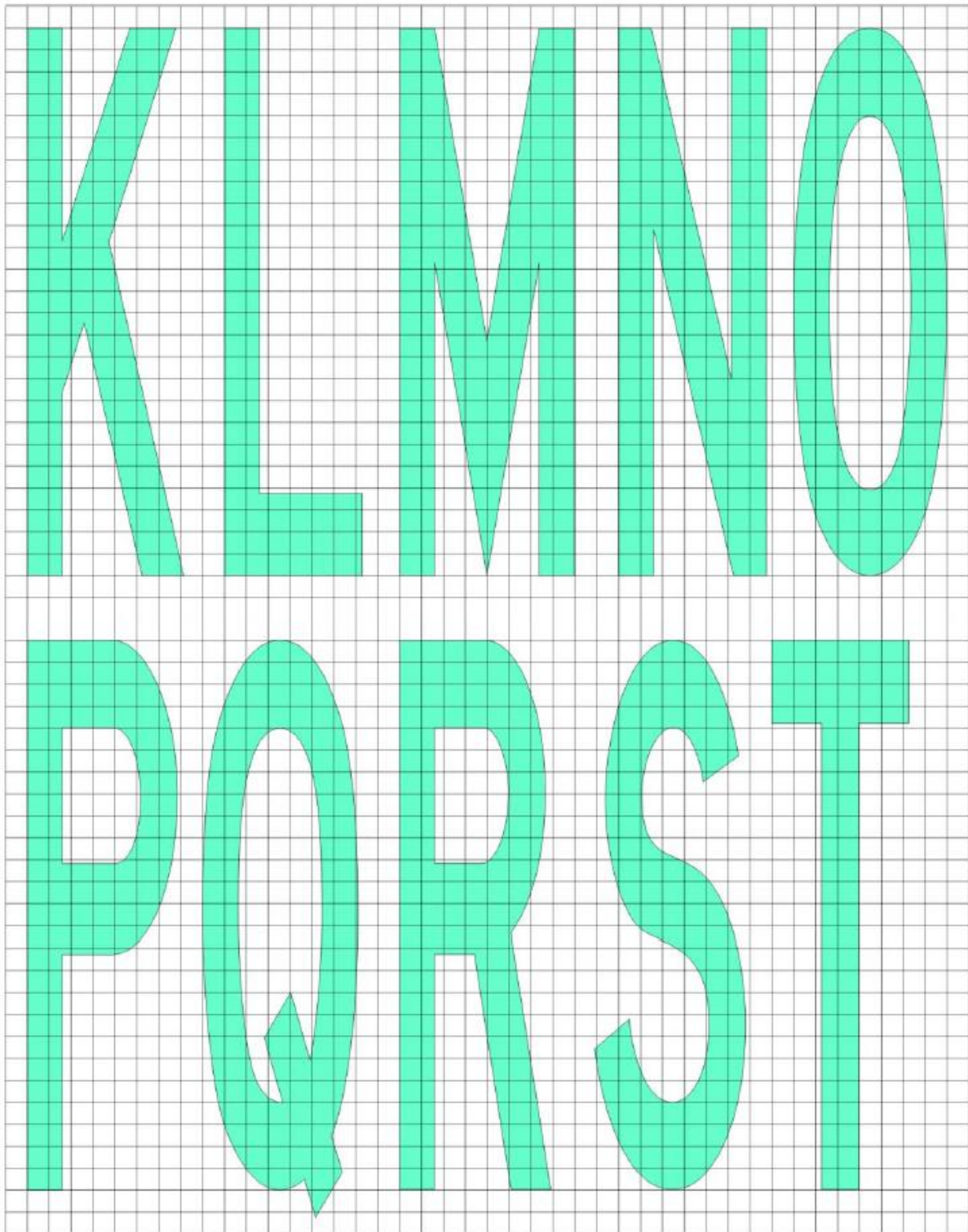
Figure L-10B. Mandatory instruction marking inscription form and proportions
