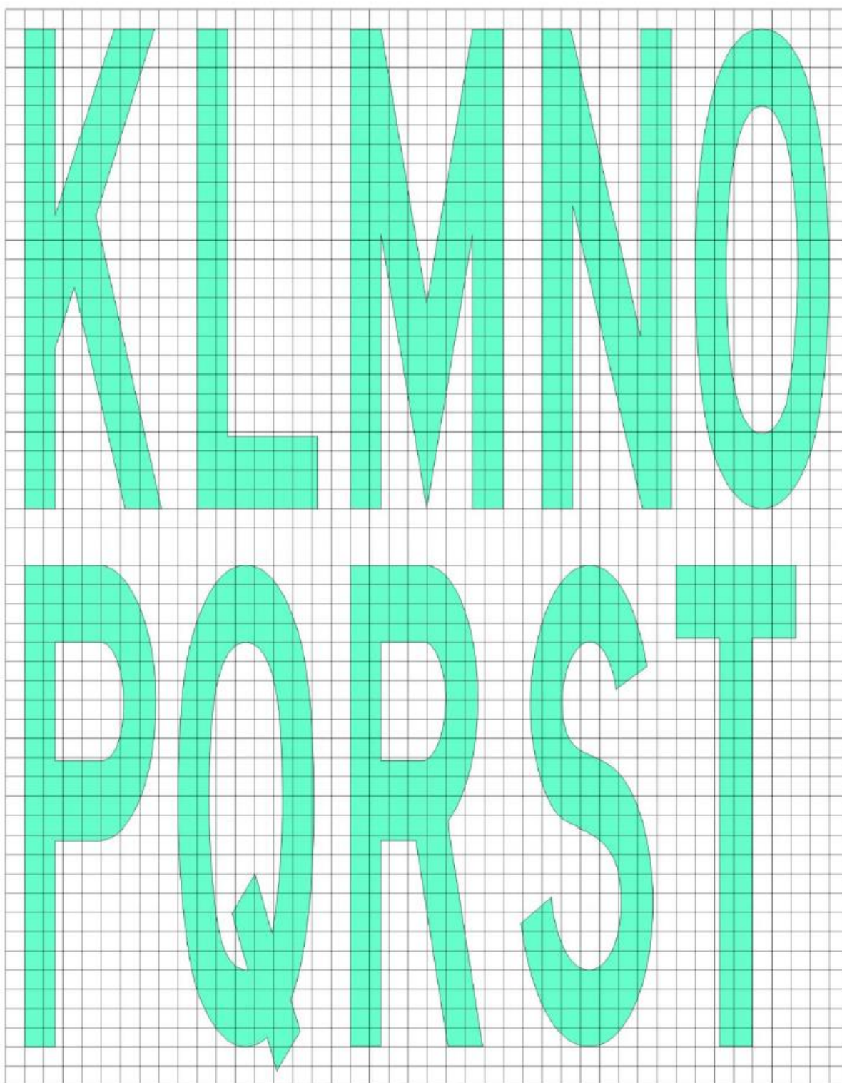
Figure L-10B. Mandatory instruction marking inscription form and proportions
