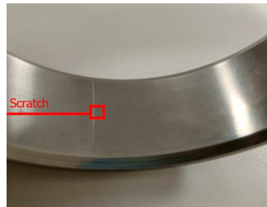
Example: Raceway of outer ring with scratch before start of testing
