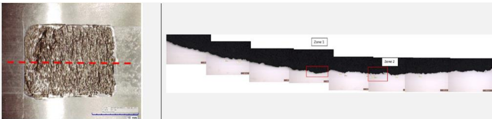
Tested outer ring (T104) with 32CDV13 at 2.9 GPa
