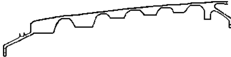
4.a - Ring Disk Drum Rotor Cross Section
