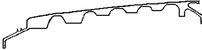
4.a - Ring Disk Drum Rotor Cross Section
