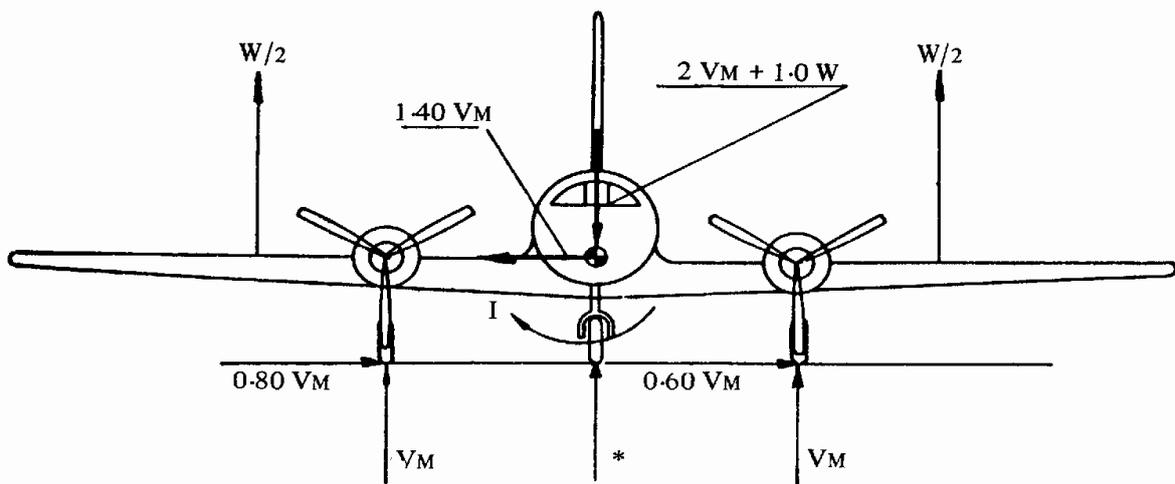
$VM$  = One-half the maximum vertical ground reaction obtained at each main gear in the level landing conditions.
