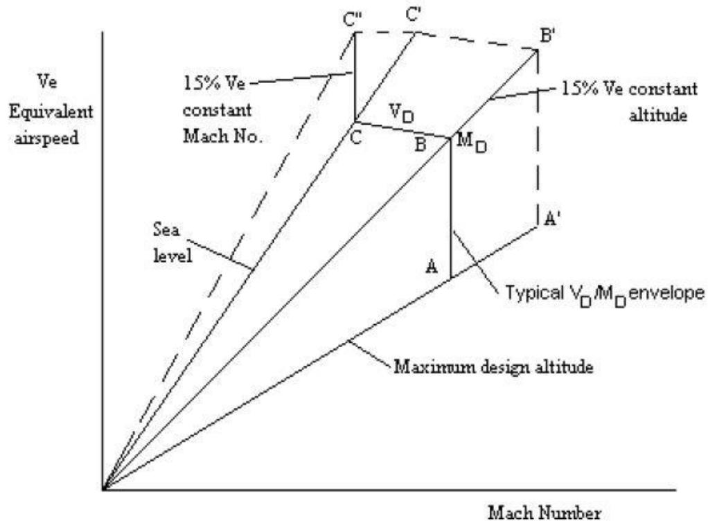
**FIGURE 1B MINIMUM FAIL-SAFE CLEARANCE ENVELOPE**
