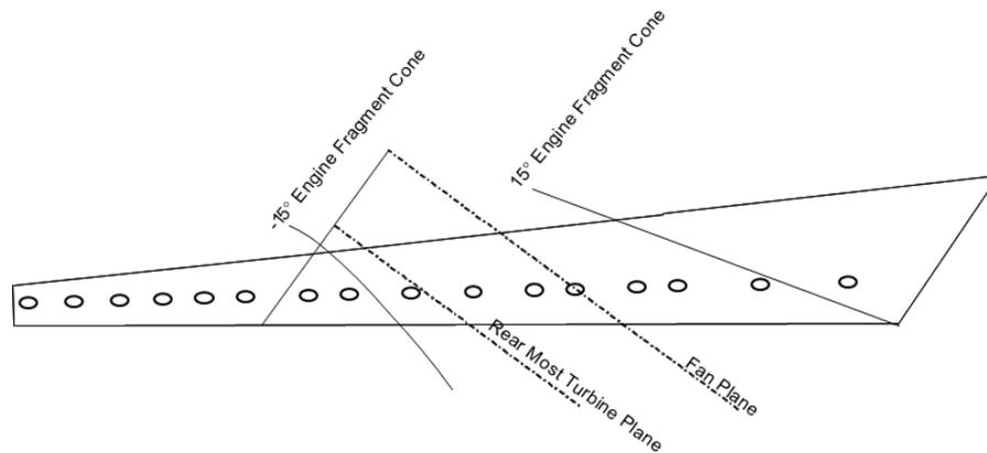
**Figure 2 — Example of the  $\pm 15$ -degree threat area representation**
