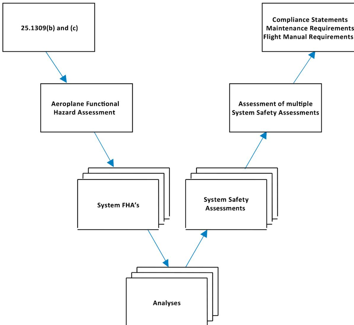
Figure A2-2: Depth of Analysis Flowchart
