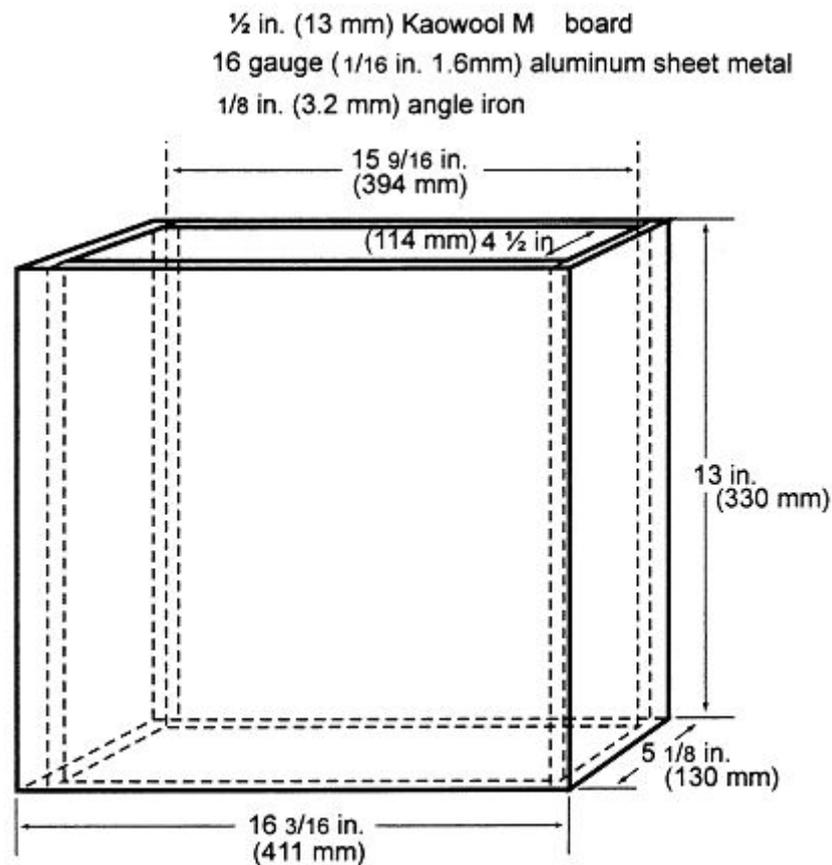
**Figure 2 - Internal Chimney**
