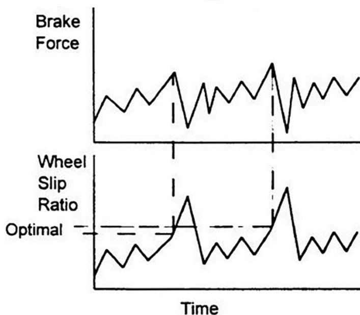
**FIGURE 6. SUBSTANTIATION OF THE OPTIMAL SLIP VALUE**
