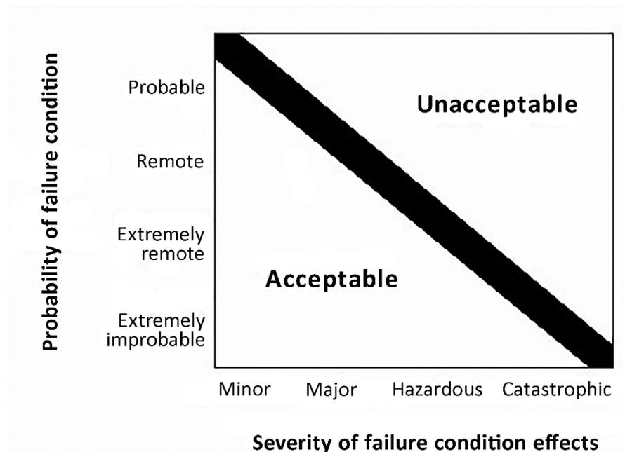
b. The safety objectives associated with Failure Conditions are described in Figure 2.
