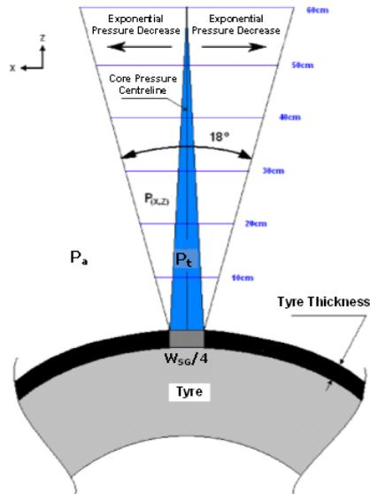
**Figure 4c – Tyre Burst Pressure Effect – Bias Tyre**
