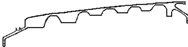
4.a - Ring Disk Drum Rotor Cross Section
