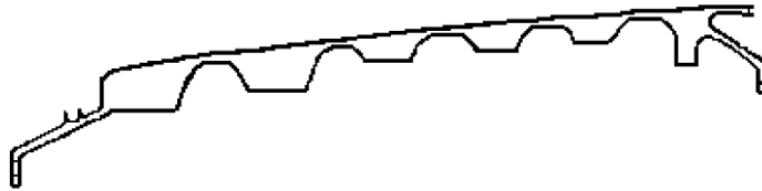
4.a - Ring Disk Drum Rotor Cross Section
