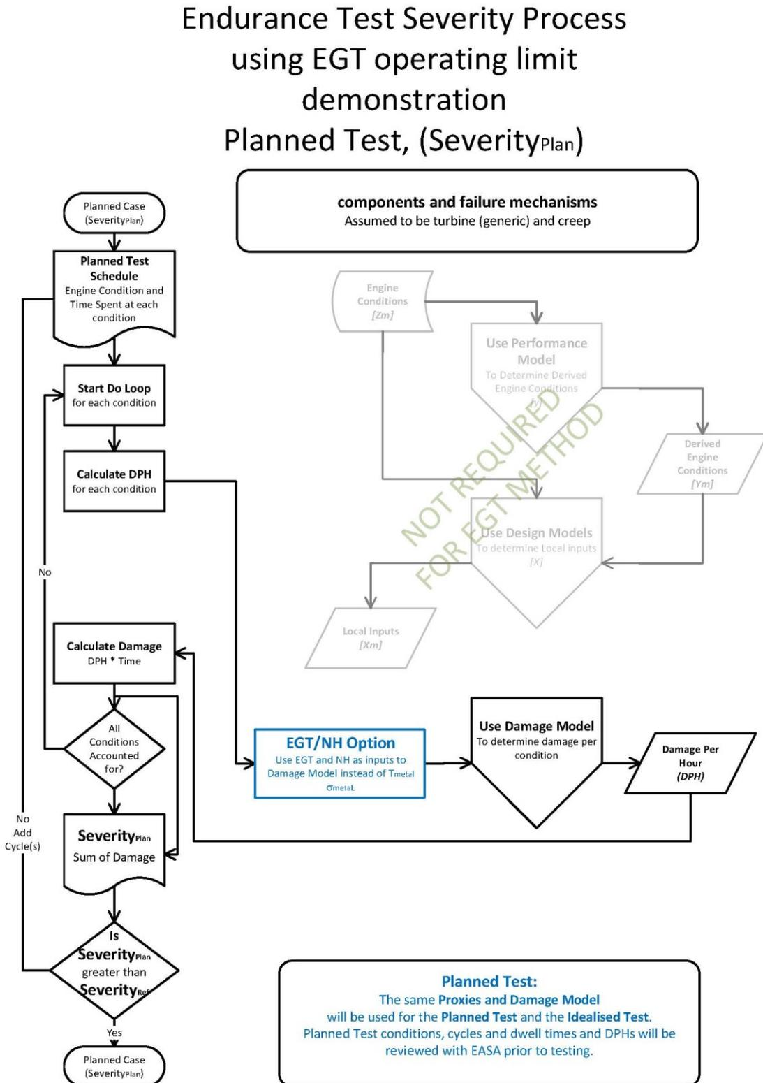
**Figure 8.10. Endurance Test Severity Process using EGT OL Demonstration – Idealised Test ( $Severity_{Plan}$ )**
