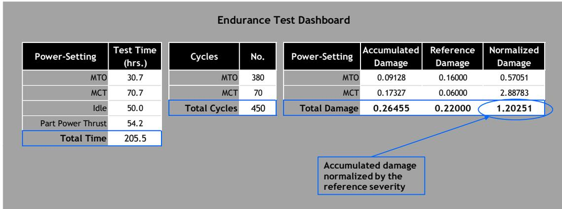
**Figure 7.6. Cumulative Severity Usage for Whole Test – first example**
