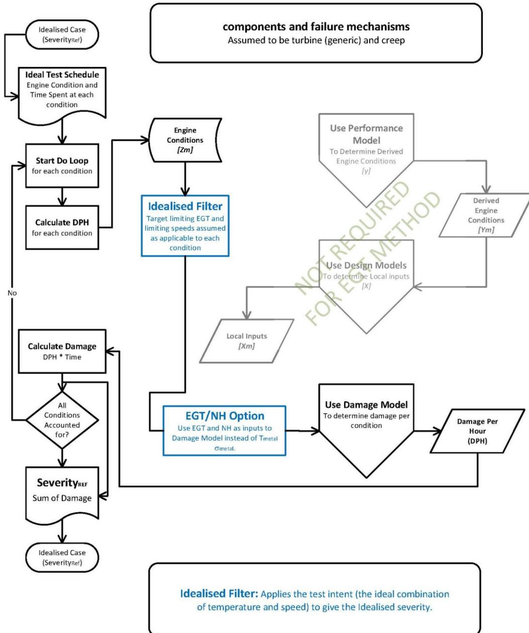
**Figure 8.9. Endurance Test Severity Process using EGT OL Demonstration – Idealised Test ( $Severity_{Ref}$ )**
