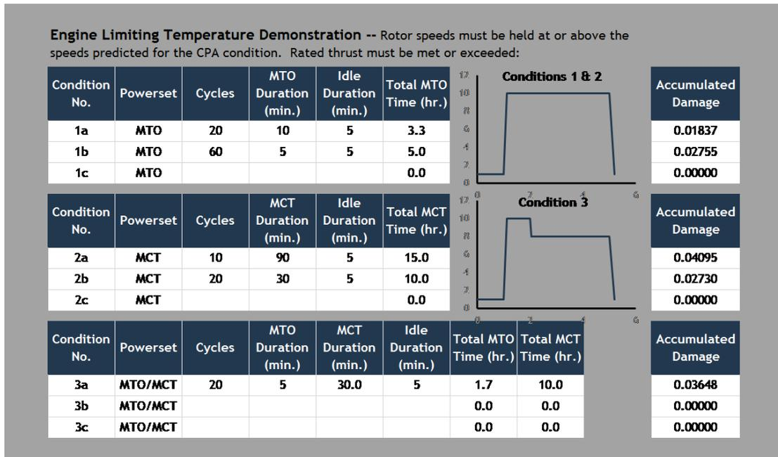
**Figure 7.4. Severity Usage for Extended Operating Periods**
