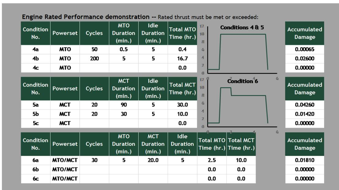
**Figure 7.5. Severity Usage for Additional Extended Conditions**
