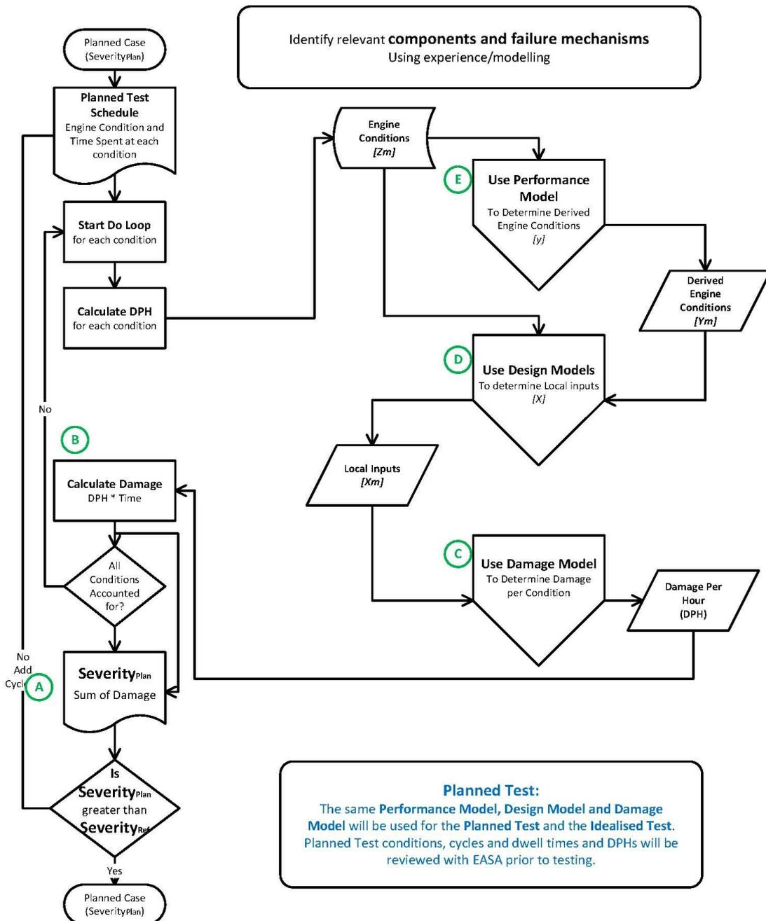
**Figure 8.4. Endurance Test Severity Process – Planned Test ( $Severity_{Plan}$ )**
