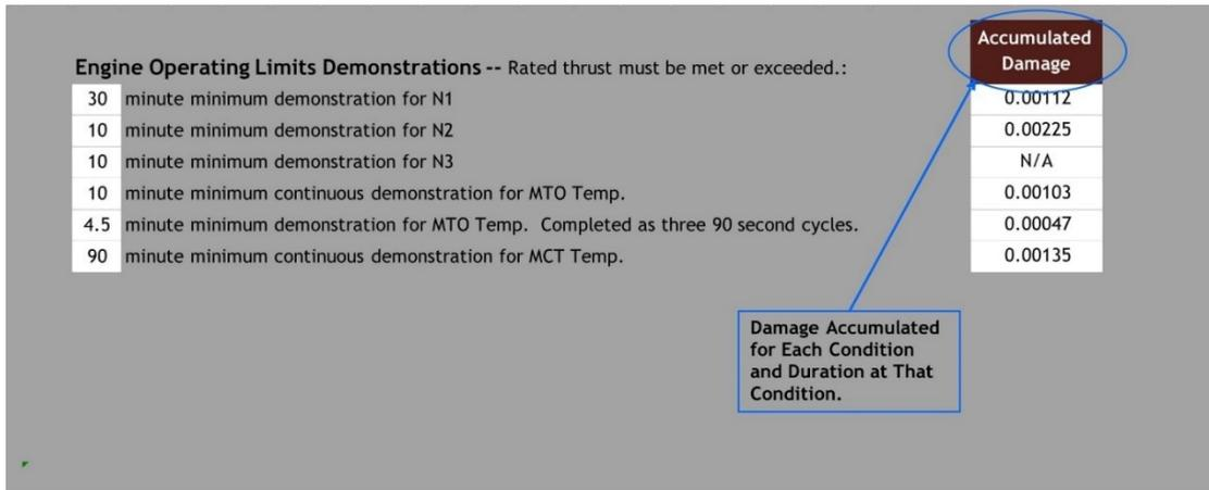
**Figure 7.2. Severity Usage for Engine Operating Limit Demonstrations**
