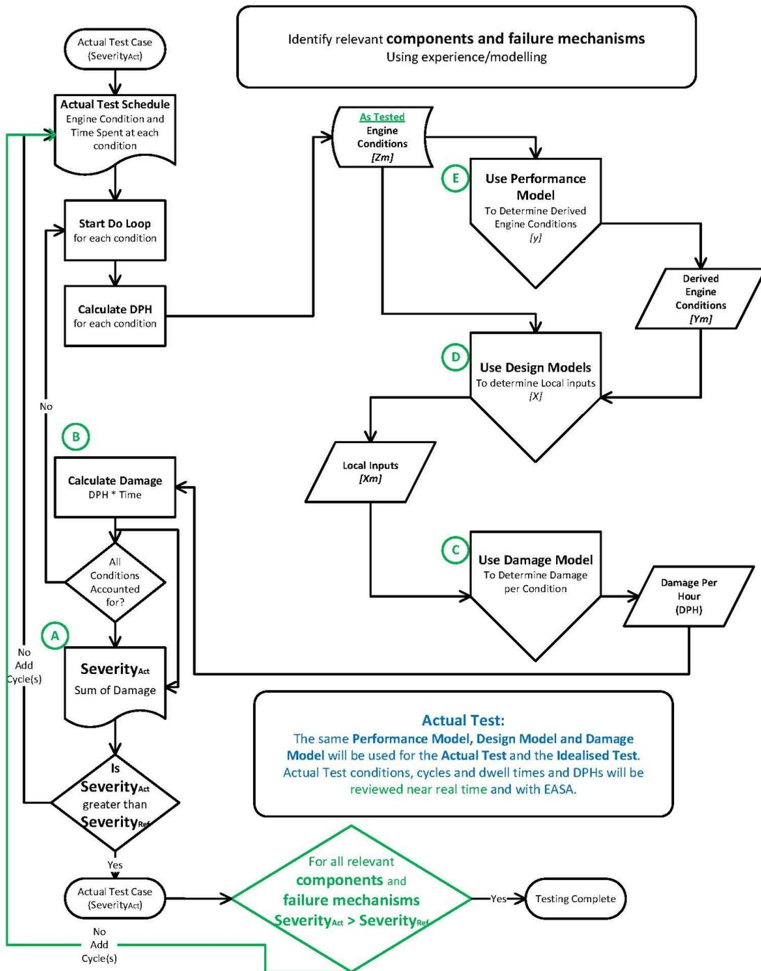
**Figure 8.5. Endurance Test Severity Process – Actual Test ( $Severity_{Act}$ )**
