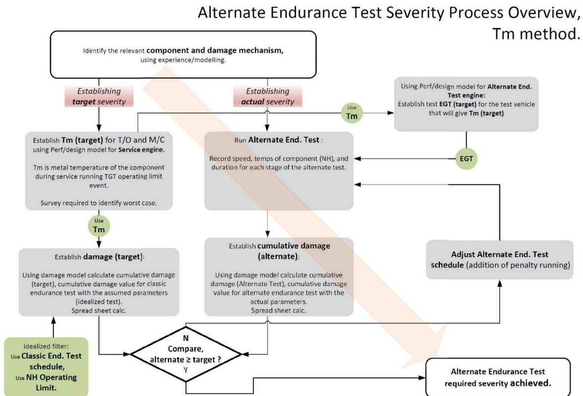
**Figure 8.1.  $T_{metal}$  method overview.**
