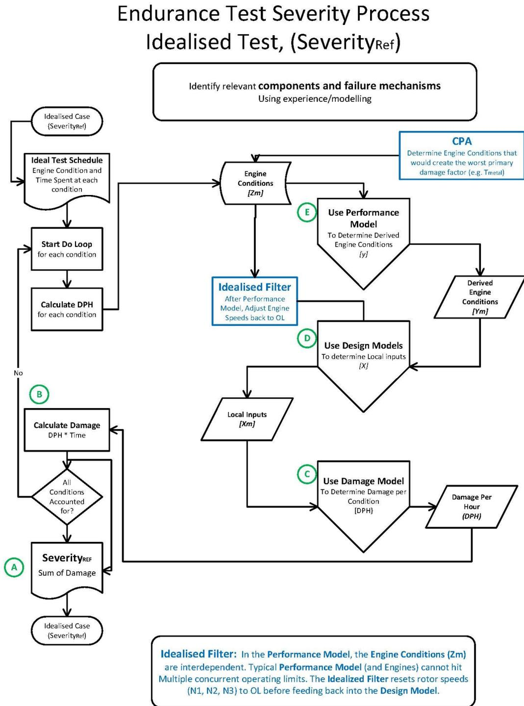
**Figure 8.3. Endurance Test Severity Process – Idealised Test ( $Severity_{Ref}$ )**
