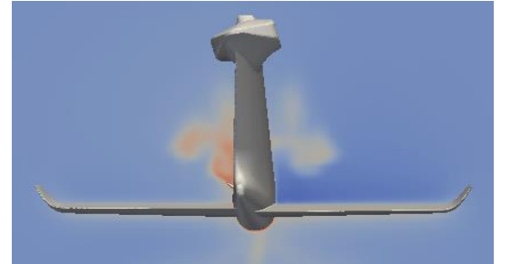
Wake propagation CS29 with HEFS pods
