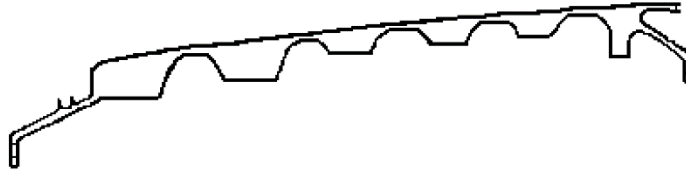
4.a - Ring Disk Drum Rotor Cross Section
