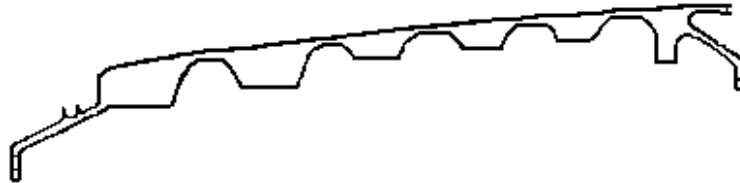
4.a - Ring Disk Drum Rotor Cross Section
