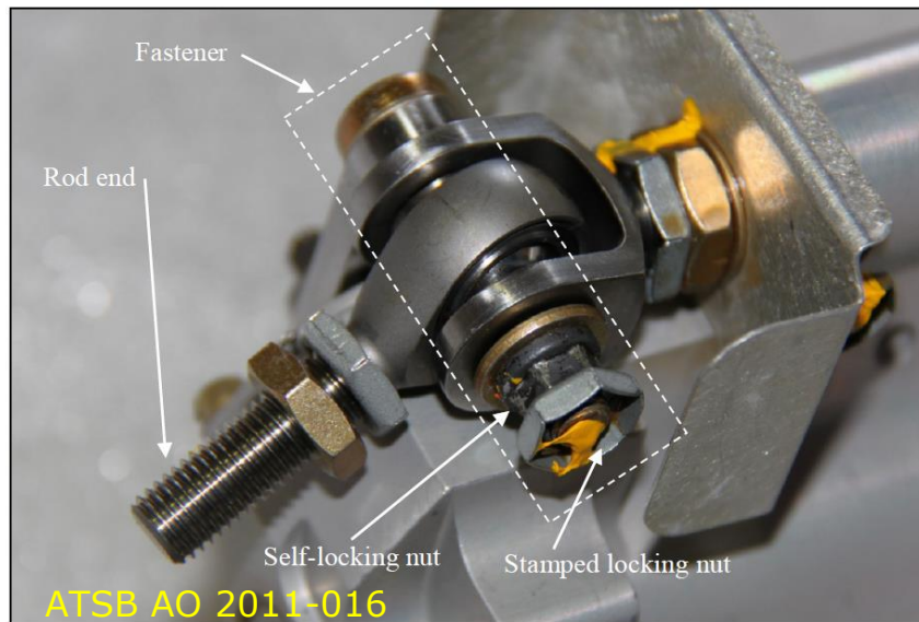
Figure 8: Lower flight control push-pull tube rod end
