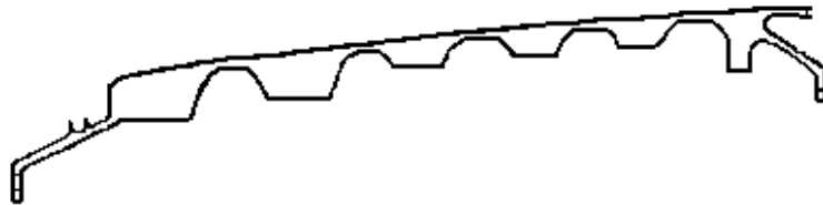
4.a - Ring Disk Drum Rotor Cross Section
