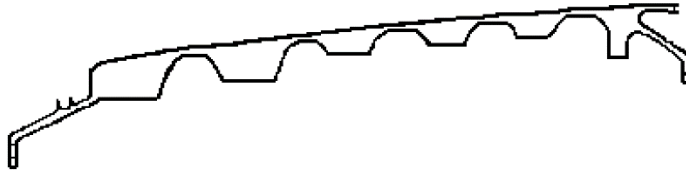
4.a - Ring Disk Drum Rotor Cross Section
