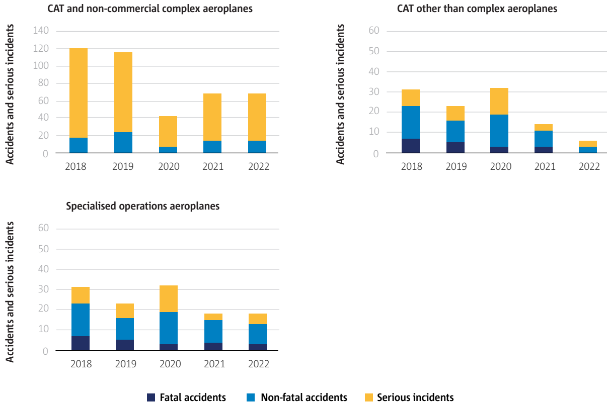
► Figure 1.3 EASA Member States accidents and serious incidents per year for CAT and non-commercial complex aeroplanes, CAT other than complex aeroplanes, and SPO aeroplanes
