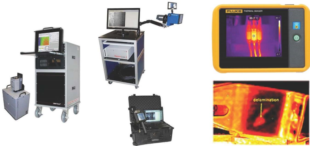
Figure 43 — Portable thermographic test equipment, potentially including an image evaluation system
