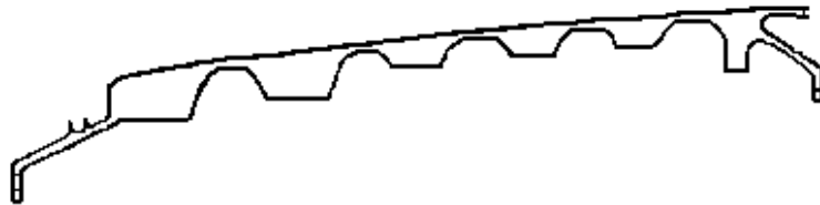
4.a - Ring Disk Drum Rotor Cross Section
