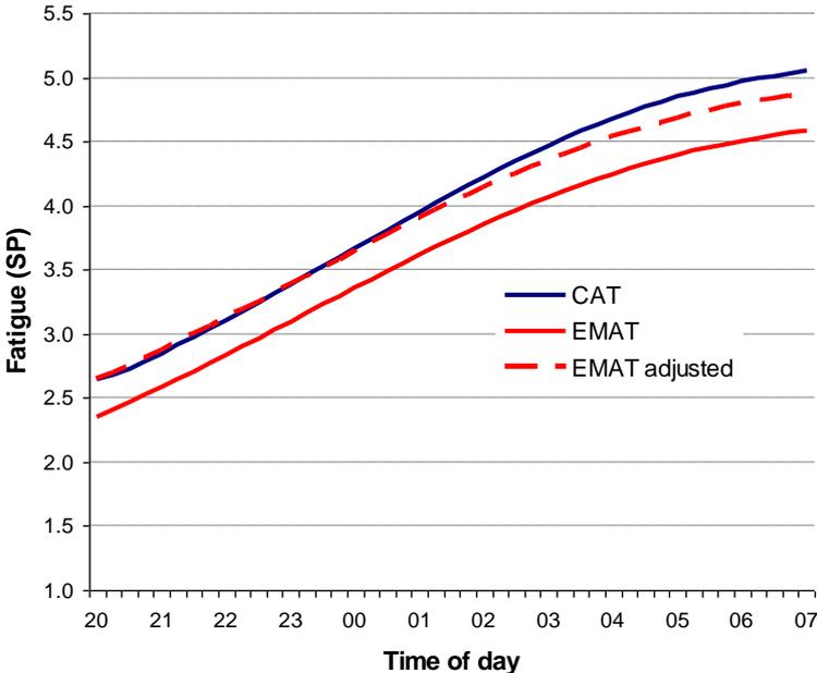
Figure 1: comparison for an 11-hour duty starting at 20:00, where the blue line corresponds to the SAFE prediction and the continuous red line to the EMAT prediction
