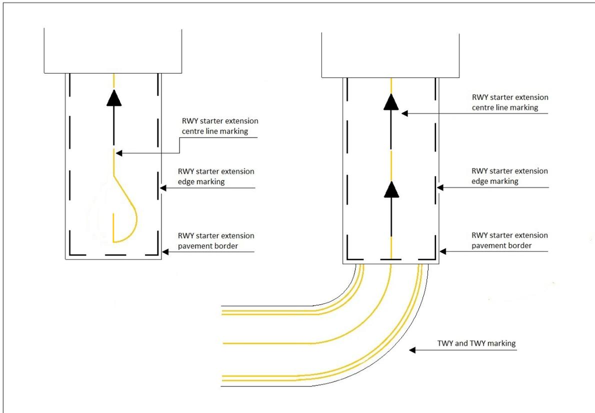
Figure L-5A. Marking of the runway starter extension
