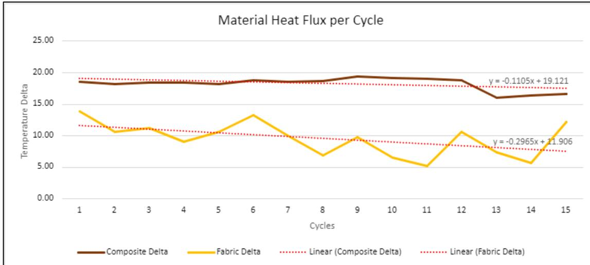
Figure 4: Material Temperature Delta per Heat Cycle and Trendlines
