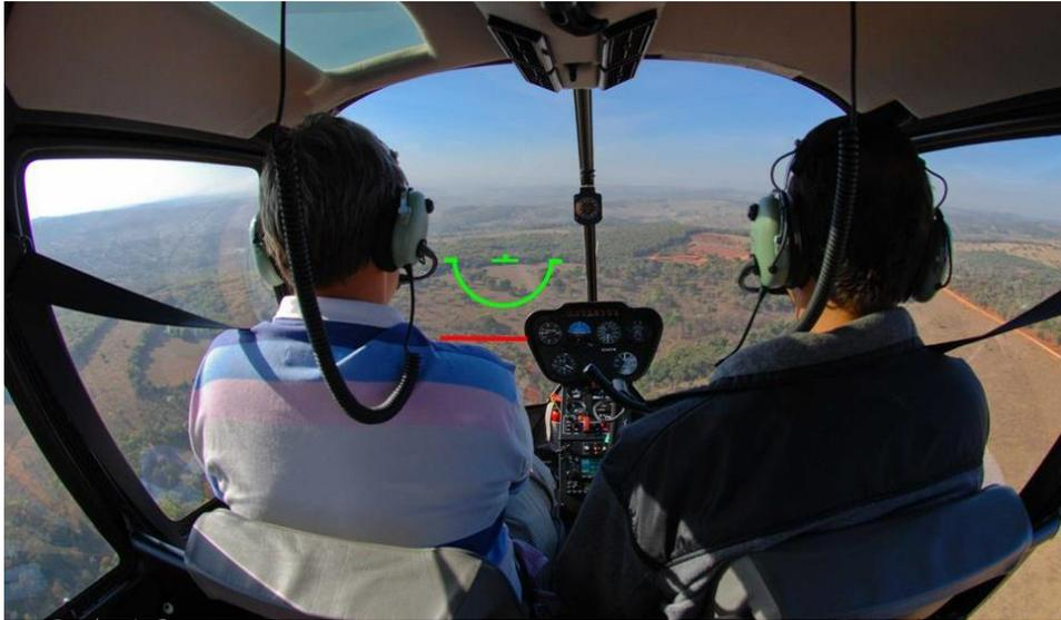
*Figure 6 Head-Up Display (HUD) of attitude recovery using the “orange peel”*
