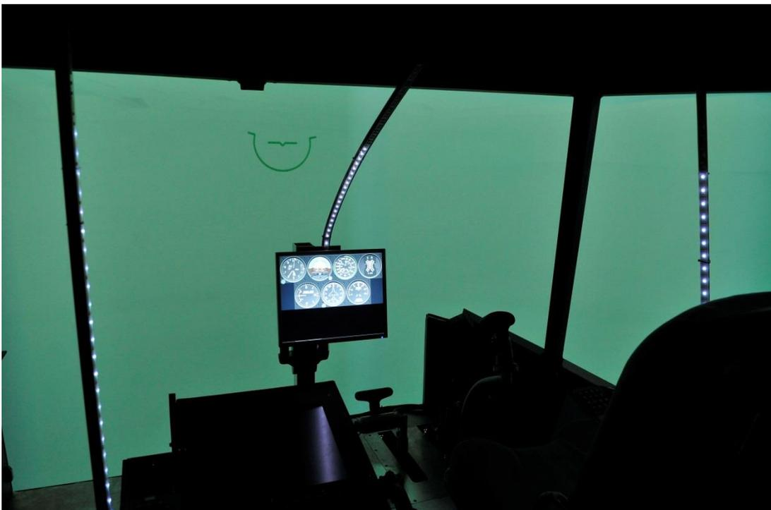
*Figure 13 HUD Orange Peel symbology (together with LED strips)*
