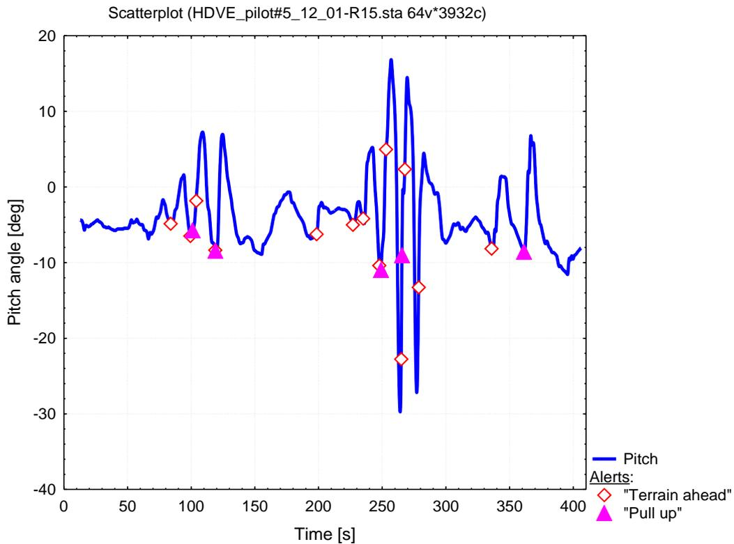
Figure 27 Pitch angle response to the HTAWS alerts during flight of Figure 26
