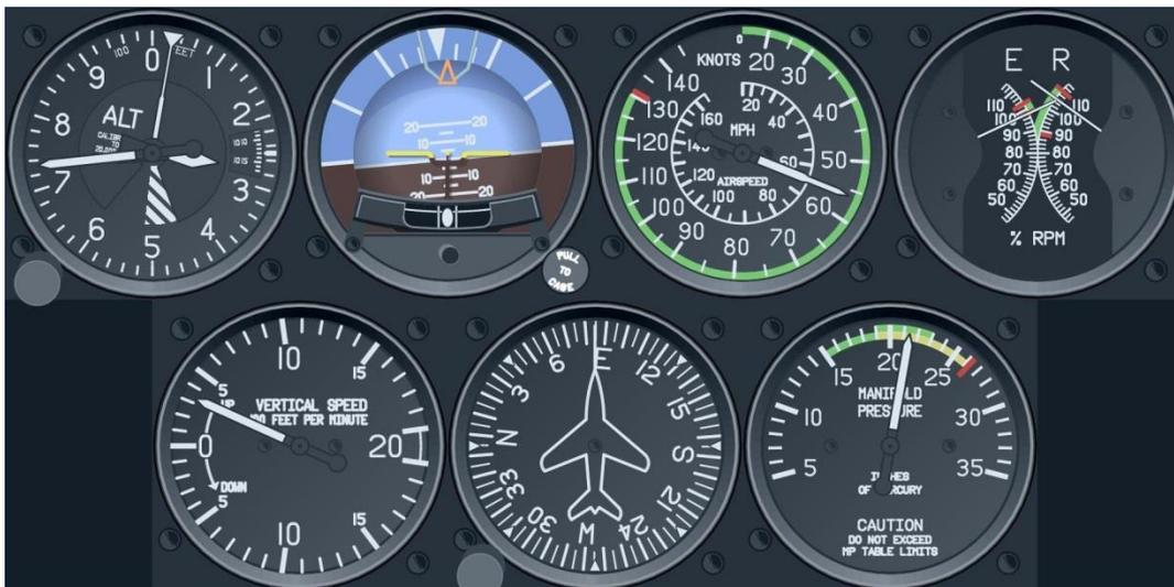
*Figure 12 Robinson R44 instrument panel to be used in the Helicopter Pilot Station. The instruments include an Attitude Director Indicator and altitude and speed dials.*
