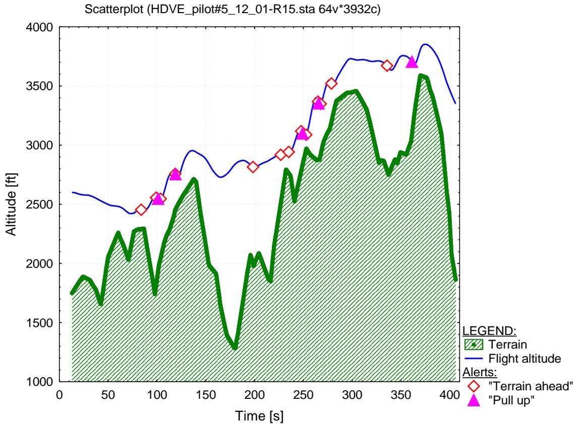
Figure 26 Altitude and alert response during flight with HTAWS in CFIT scenario
