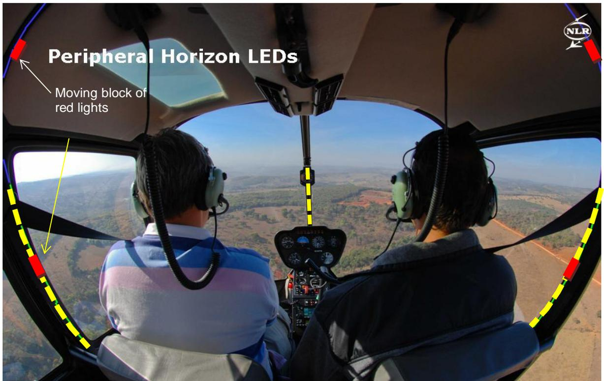
*Figure 8 Lights (LEDs) mounted in the peripheral view of the pilot*
