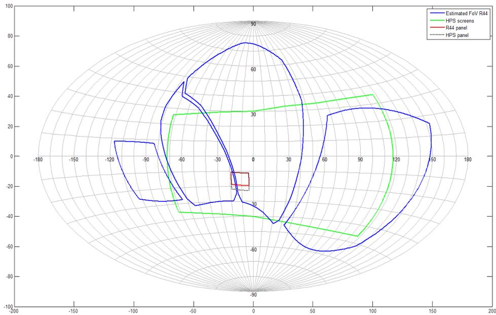
*Figure 11 Optical field-of-view from the pilot's eye reference point in the HPS, with the new 19" instrument panel, relative to the R44 helicopter; HPS rotated 21.75° left relative to centerline*
