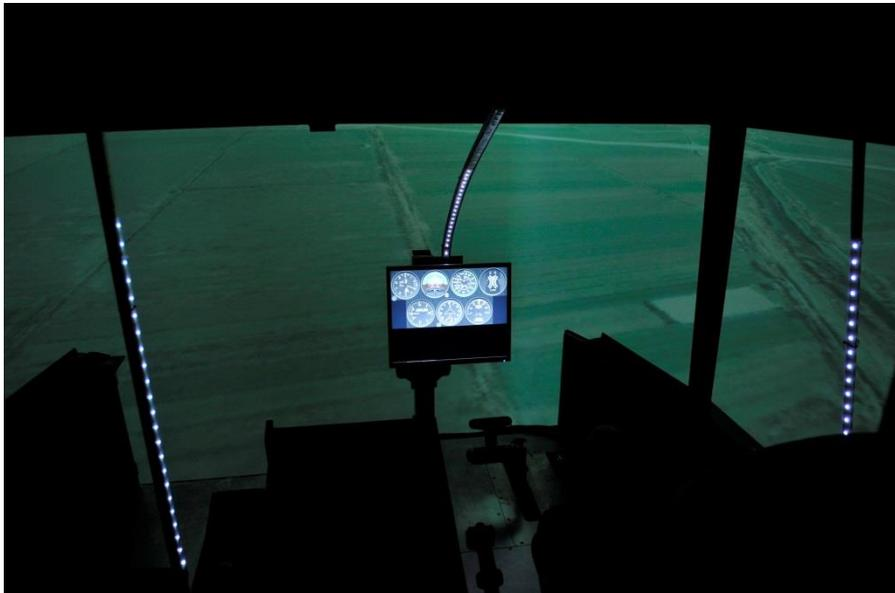
*Figure 14 LED concept of three strips/poles in the cockpit*
