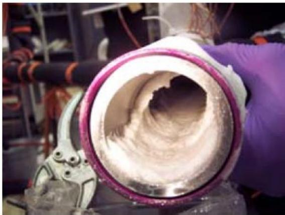
(a) Ice in a hose at the rear of the strut.
