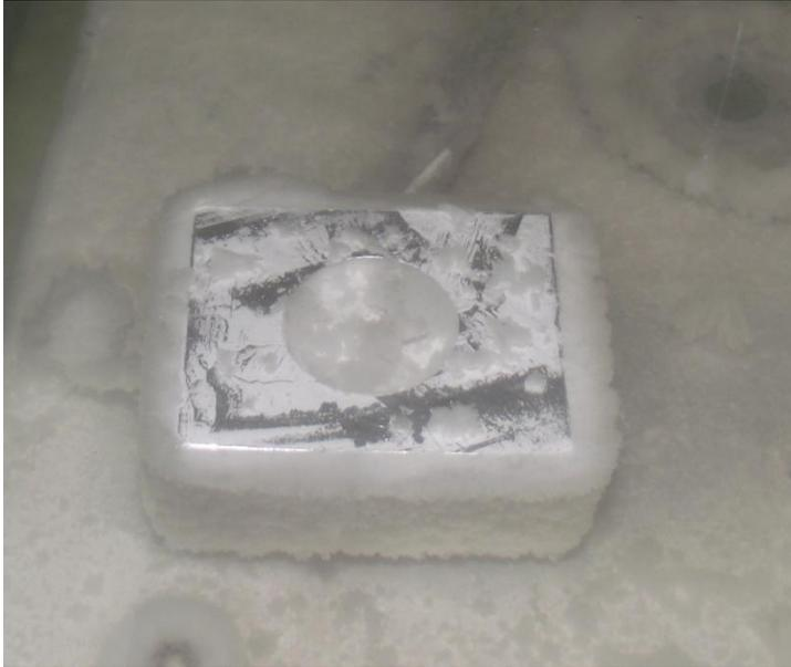
(a) The ice layer thickness at the top of the vertical surfaces could be seen clearly from the picture.
