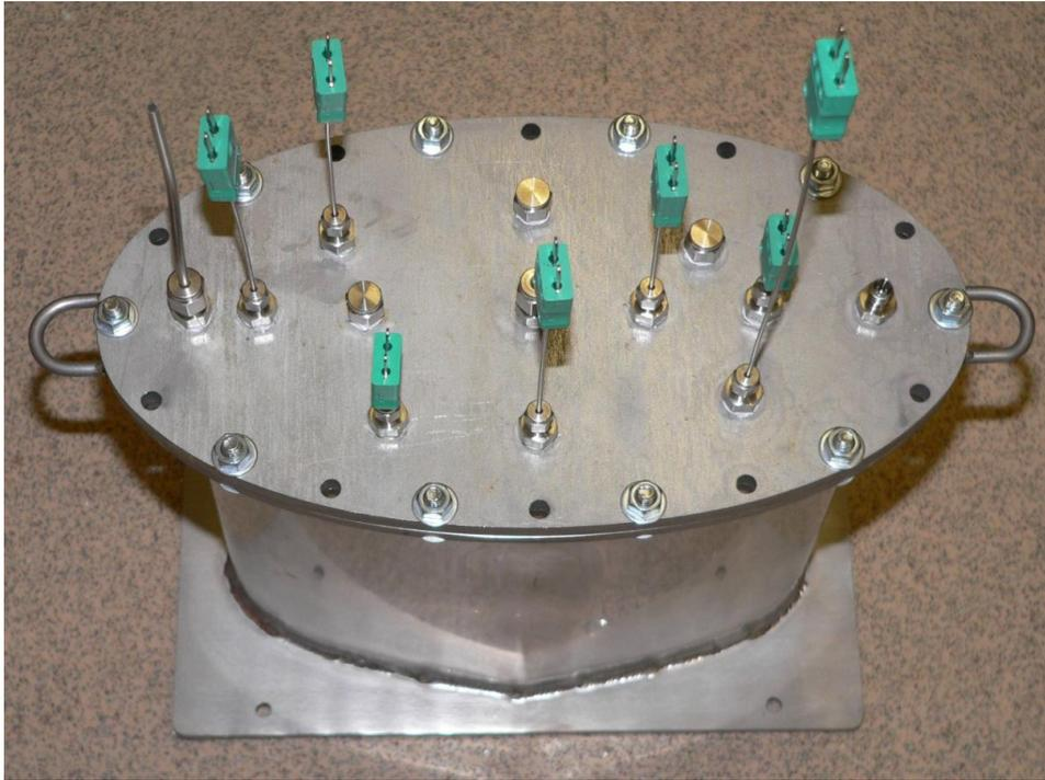
**Plate 18     Jorin ViPA coupled to fuel container inside freezer. The port connector facilitates fluid and thermocouple connections inside the freezer. Data from the system is displayed on a remote computer**
