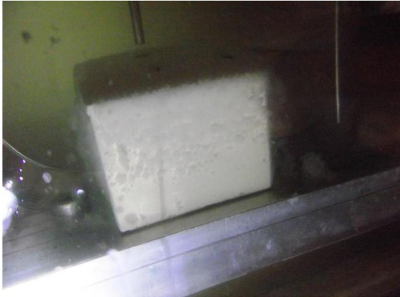
**Figure 17** Ice accreted on a vertical composite surface of SB3 (composite) in Test #1.
