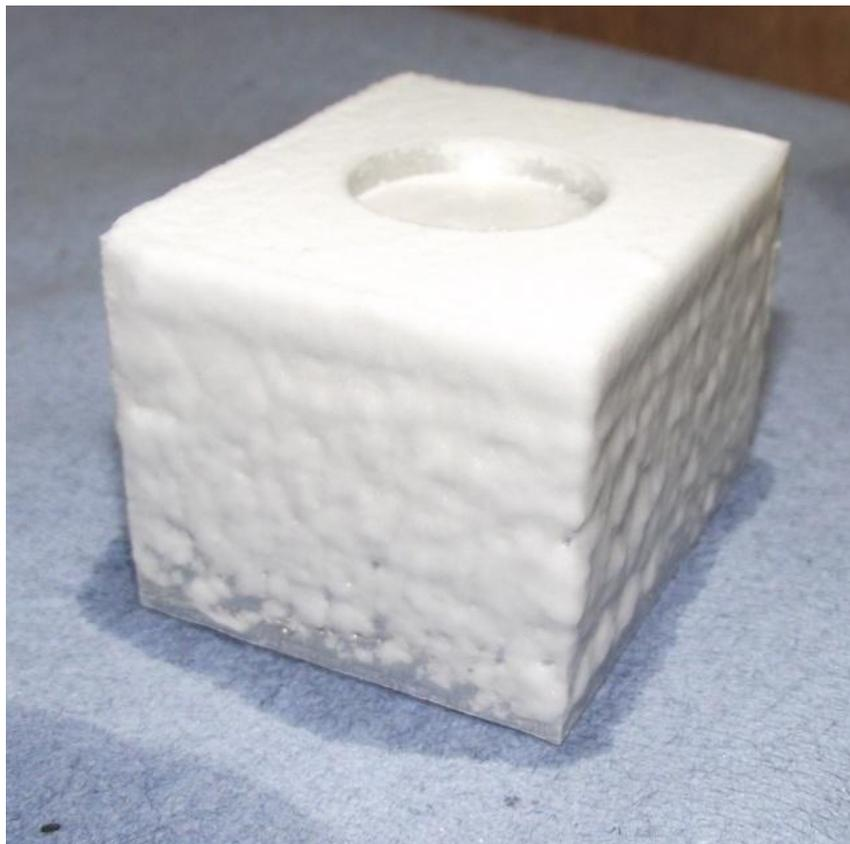
(c) Ice covered area on the vertical surfaces. Thinning of the ice layer towards the foot of the vertical surfaces is observed.
