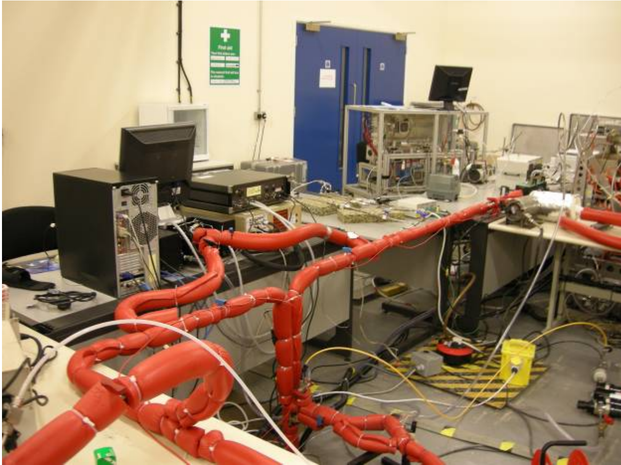
Rear of the LII 200 Instrument with the heated gas sampling lines and connections shown.
