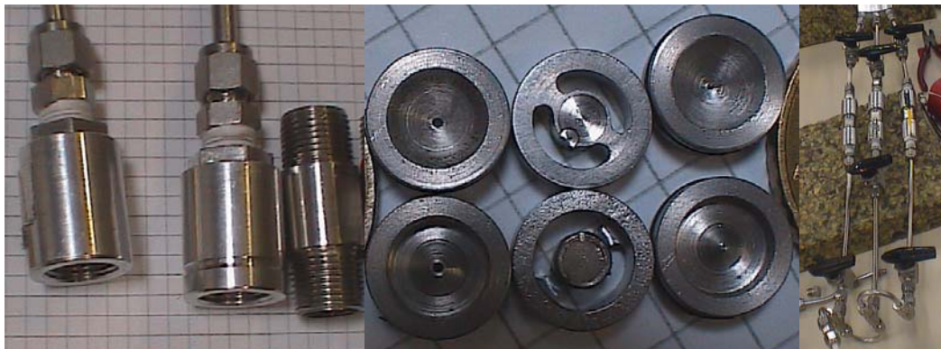
Figure 1 Two stages mini-impactor (left panel: holder; middle panel: nozzles and supports of TEM grids, right panel: experimental set-up)
