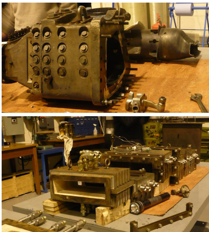
Figure 3. Combustor pressure casing (top, front), combustor can (top back), and HES components (bottom).
