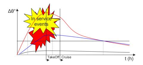
The Monte-Carlo method averaging out a critical area related to on ground situation with heat input into the tanks. Red line and blue line might result in same flammability exposure using FAA Monte Carlo flammability exposure model, however redline results in critical high flammability in certain ground conditions.
