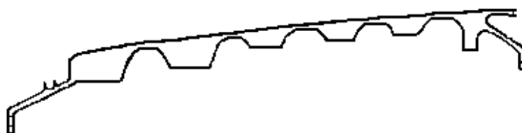
4.a - Ring Disk Drum Rotor Cross Section
