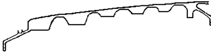
4.a - Ring Disk Drum Rotor Cross Section
