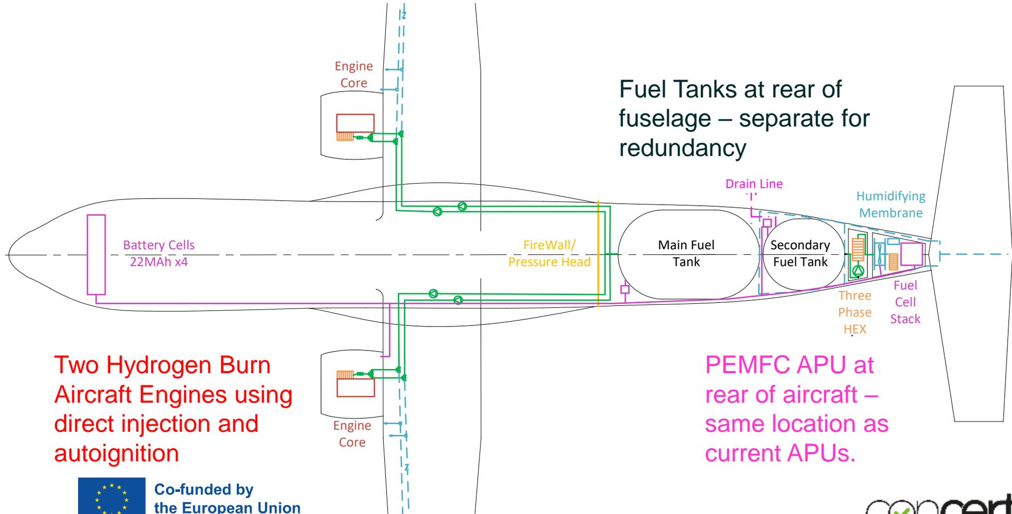
Two Hydrogen Burn Aircraft Engines using direct injection and autoignition
