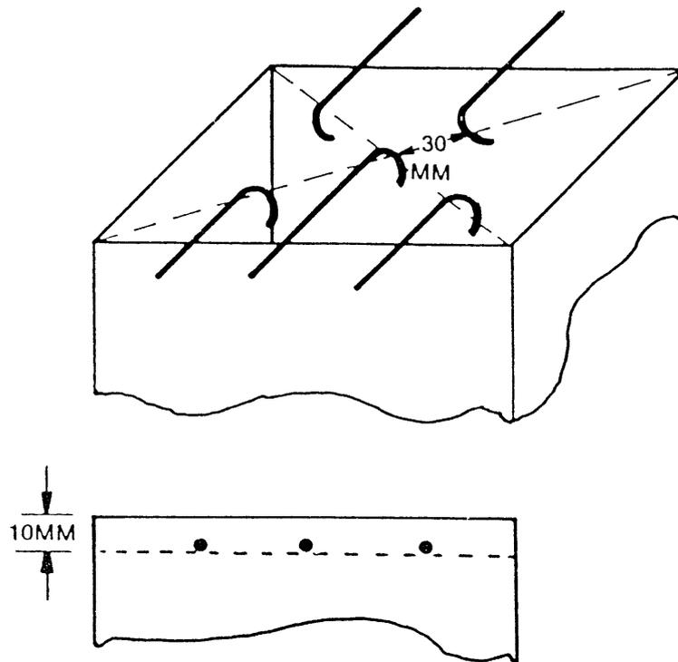
FIGURE 5. THERMOCOUPLE POSITION
