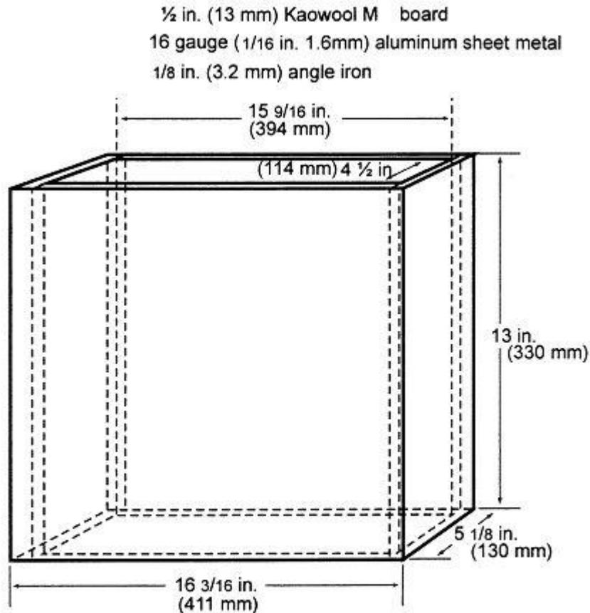
Figure 2 - Internal Chimney
