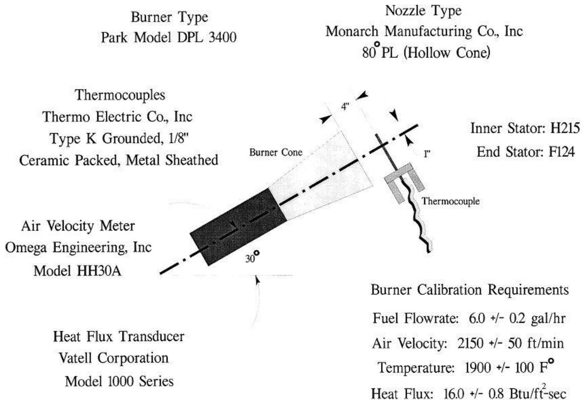
Figure 8 – Burner Information and Calibration Settings
