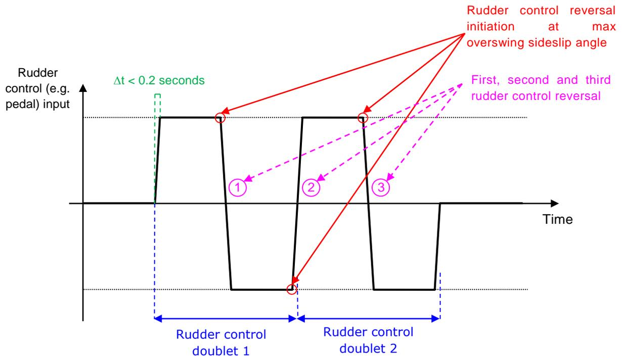
Figure 1: Illustration of the cockpit rudder control inputs
