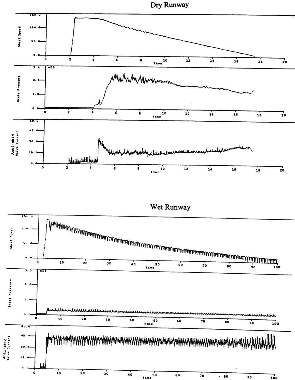
**FIGURE 3. ANTI-SKID SYSTEM RESPONSE CHARACTERISTICS Fully Modulating System**
