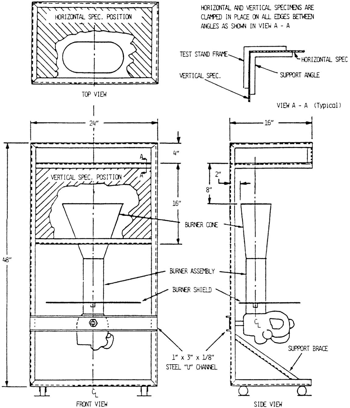
HORIZONTAL AND VERTICAL SPECIMENS ARE CLAMPED IN PLACE ON ALL EDGES BETWEEN ANGLES AS SHOWN IN VIEW A - A
