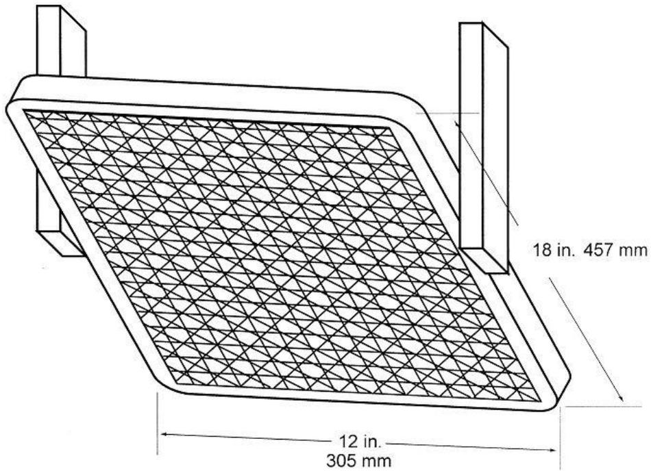
Figure 3b – Air Propane Radiant Panel
