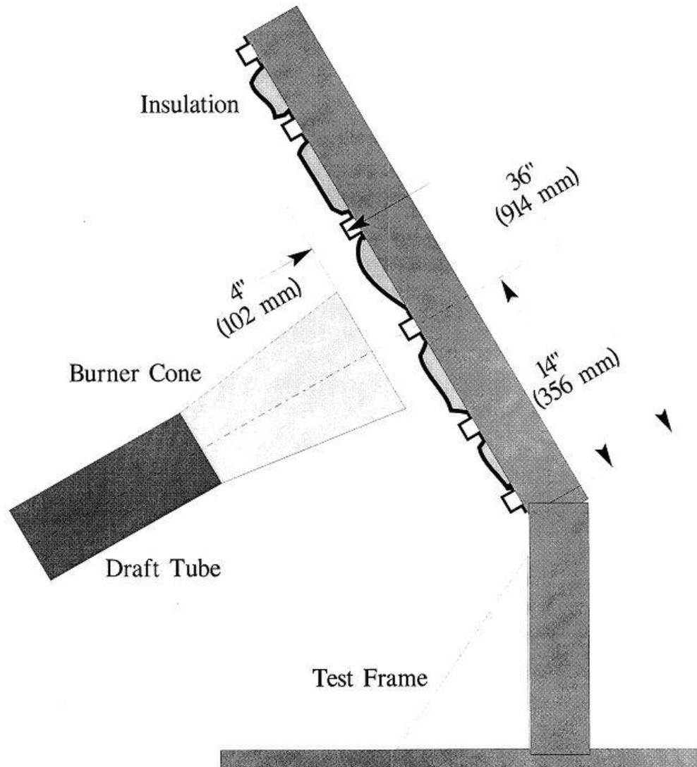
Figure 2 – Burnthrough Test Apparatus
