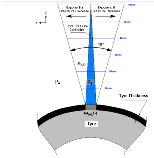
Figure 4c – Tyre Burst Pressure Effect – Bias Tyre
