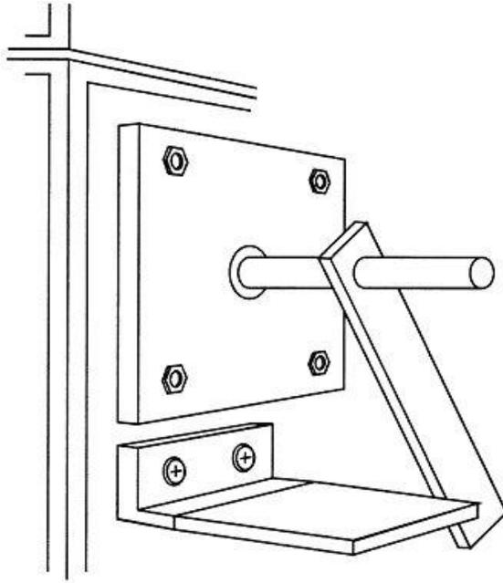
Figure 8 - Propane Burner Stop
