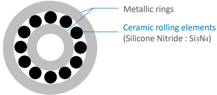
How ceramic rolling elements are produced ?
