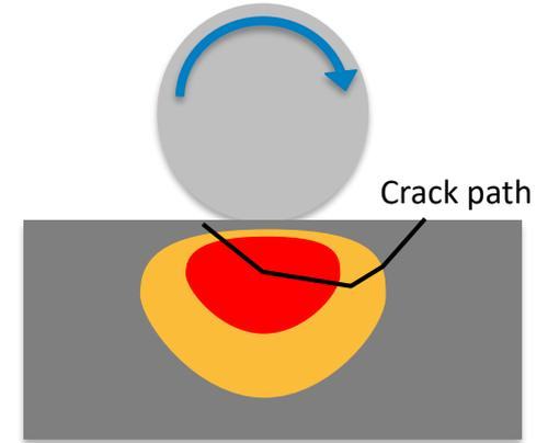
**Failure case 2:** However, the combination of RCF and significant body stresses (e.g. bending of the race) can lead to **crack through the race** (Threshold criteria not fully characterised. Topic of research)
