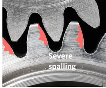
Effects: Transfer of load, etc, may no longer be ensured ? Further effects on other parts?
