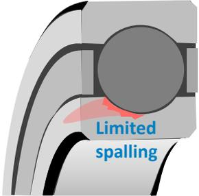
Effects: Could result in a loss of function if requiring very precise internal geometry OR if debris can remain trapped and result in jamming
