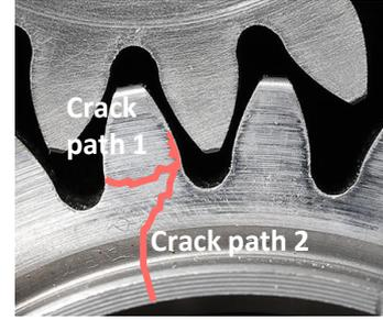
Cause: Usually only caused by initial spalling.
