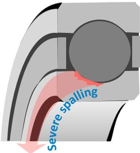
Effects: Transfer of load, adequate support, alignment, etc, may no longer be ensured ? Further effects on other parts?
