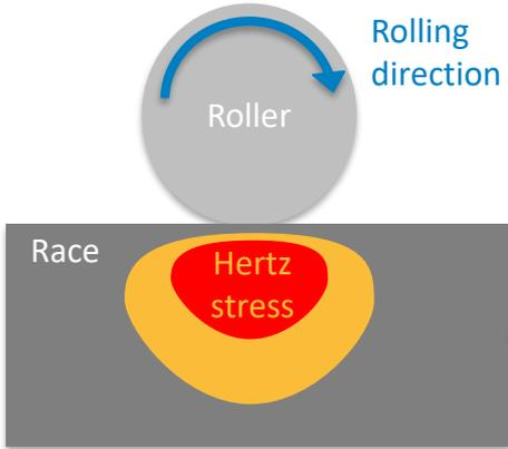
**Failure case 1:** RCF will typically lead to cracks returning to the surface lead to the release of particles, i.e. **spalling**.
