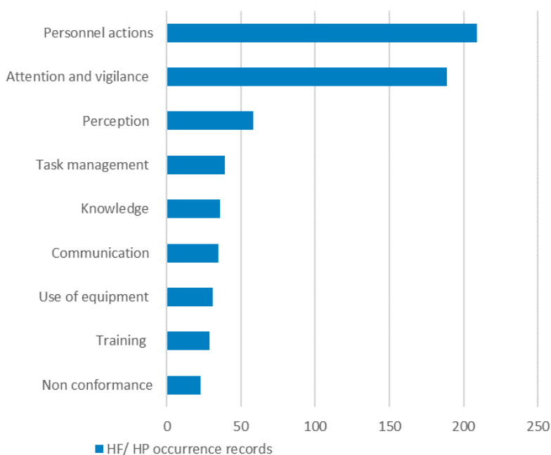
Appendix 2 Figure 7 Detailed HF/HP event codes by number of occurrences involving large aeroplanes and aeroplanes with a mass group greater than 5 700kg conducted NCC
