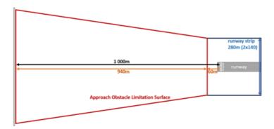
In accordance with point (e) of AMC2 ADR.OPS.B.005(b), the assessment near an aerodrome should consider significant portions underneath the standard approach and departure routes within a 8-km radius from the aerodrome reference point.
