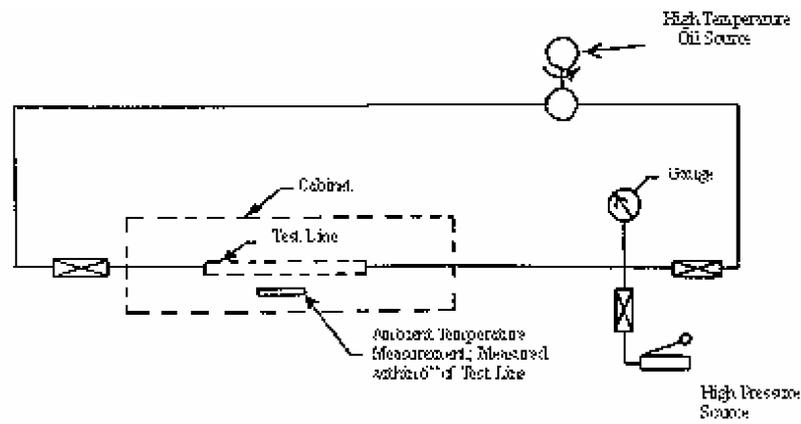
Typical Setup for High Temperature Pressure Testing
