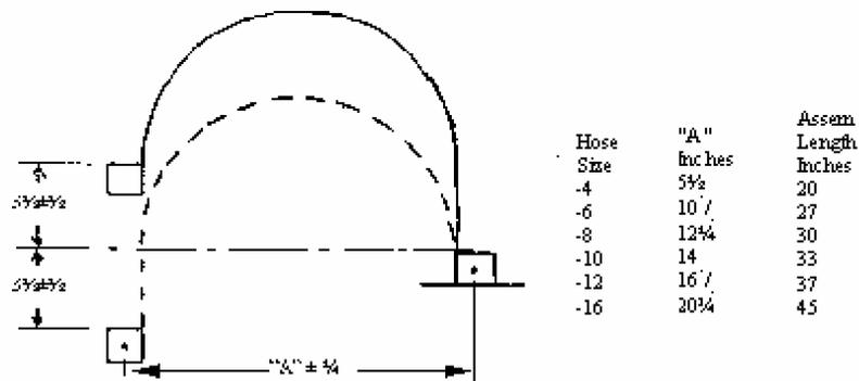
Assembly Flex Test Setup
