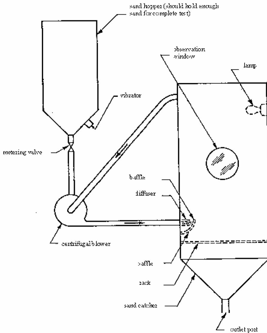
Figure 1. Schematic Sand Test Arrangement (Ref. Section 7.8)
