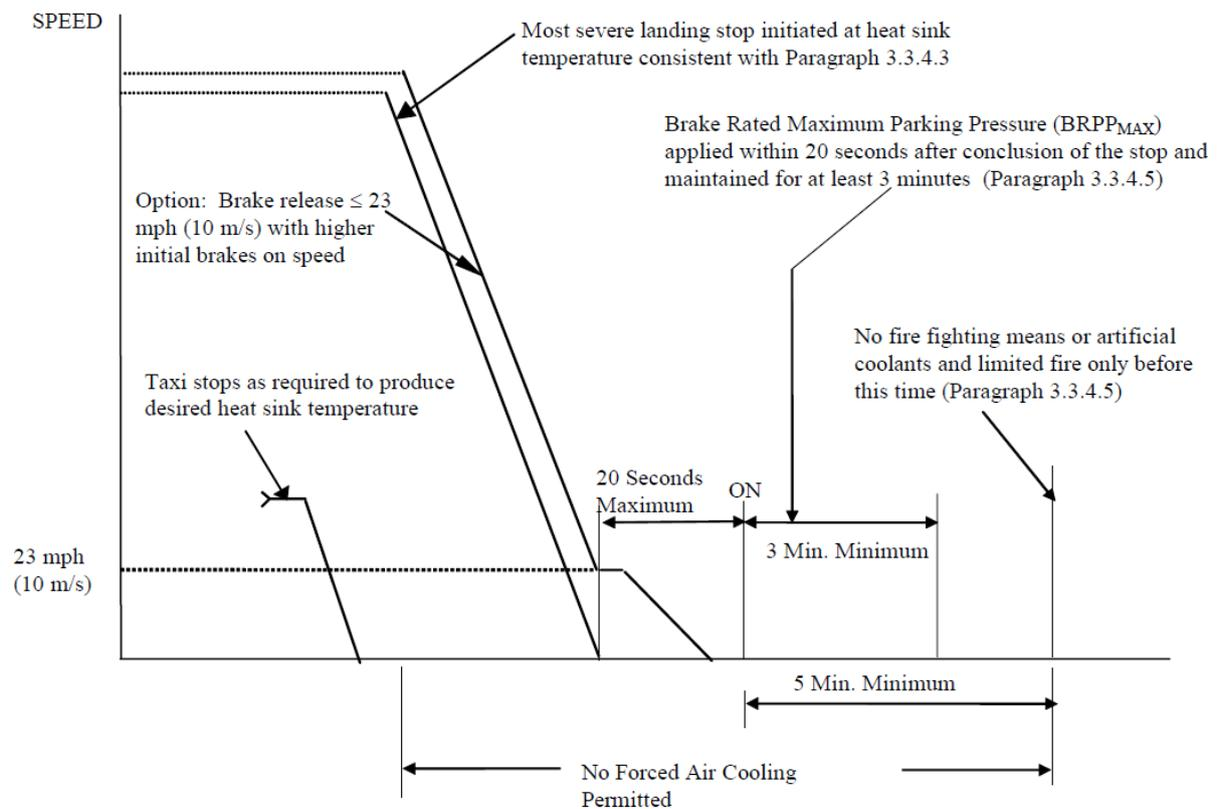
Figure 3-2. Most Severe Landing-Stop, Park Test Sequence
