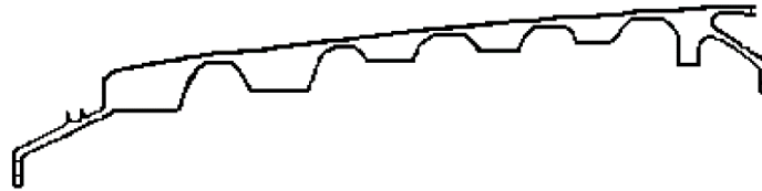
4.a - Ring Disk Drum Rotor Cross Section
