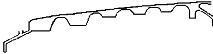
4.a - Ring Disk Drum Rotor Cross Section
