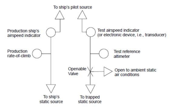
Figure 6 Trapped Static Source Schematic
