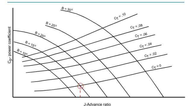
Figure 17–2 PROPELLER COEFFICIENTS
