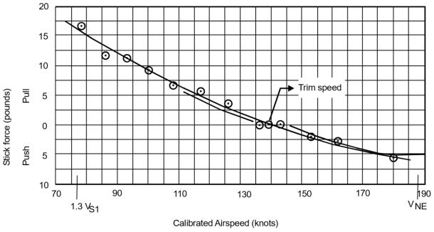
Figure 72–1 STATIC LONGITUDINAL STABILITY PLOT (CRUISE CONDITION)
