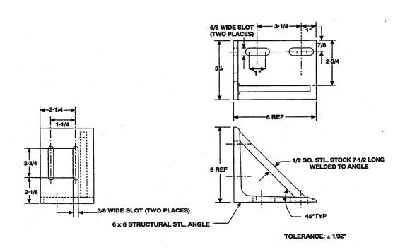
FIGURE No. 6 SUPPORT BRACKET LUMBER TEST FIXTURE
