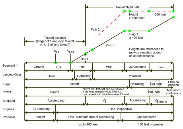
NOTE: The en route takeoff segment usually begins with the aeroplane in the en route configuration and with maximum continuous thrust, but it is not required that these conditions exist until the end of the takeoff path when compliance with 23.67(c)(3) is shown. The time limit on takeoff thrust cannot be exceeded.
