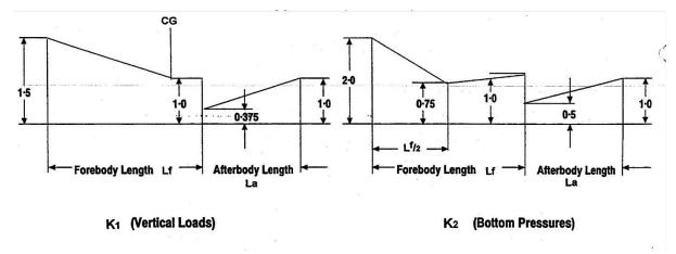
FIGURE 2. Hull station weight factor
