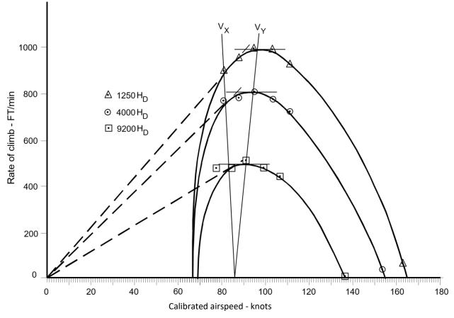
Figure 25–2 RATE OF CLIMB VS. AIRSPEED
