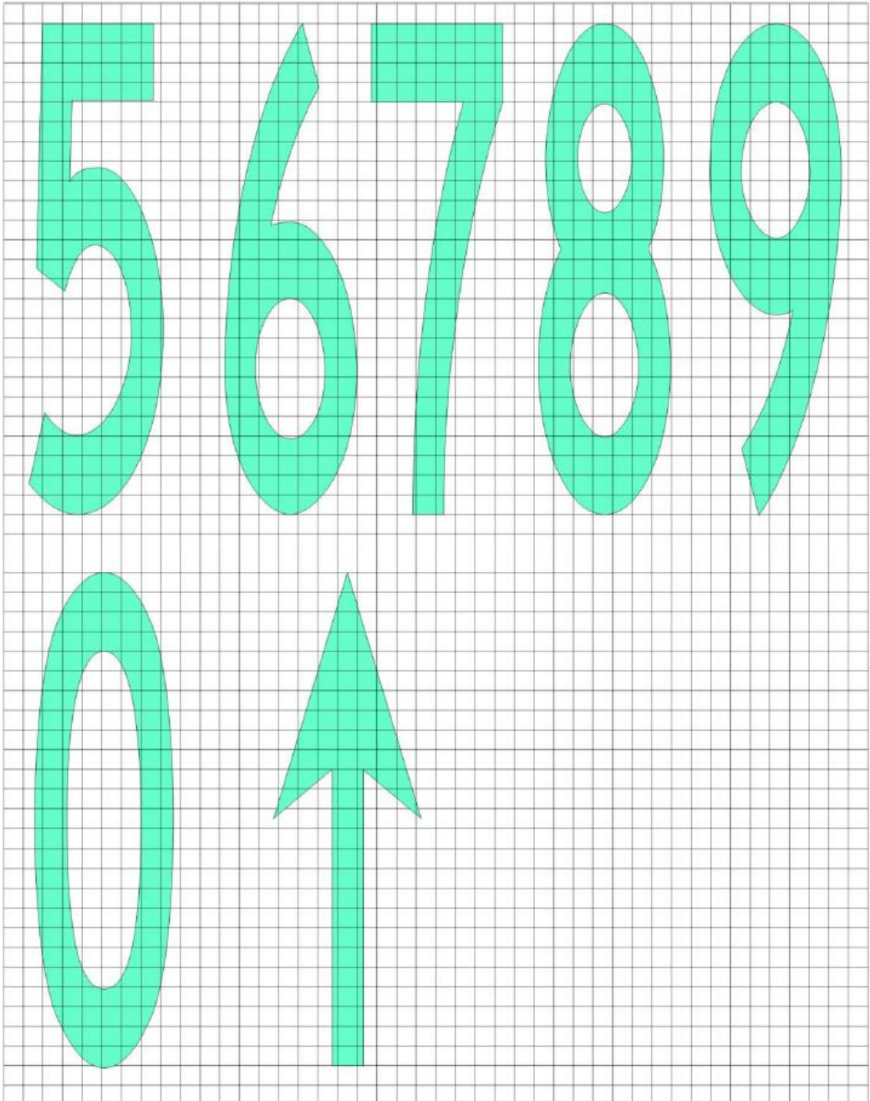
Figure L-10D. Mandatory instruction marking inscription form and proportions
