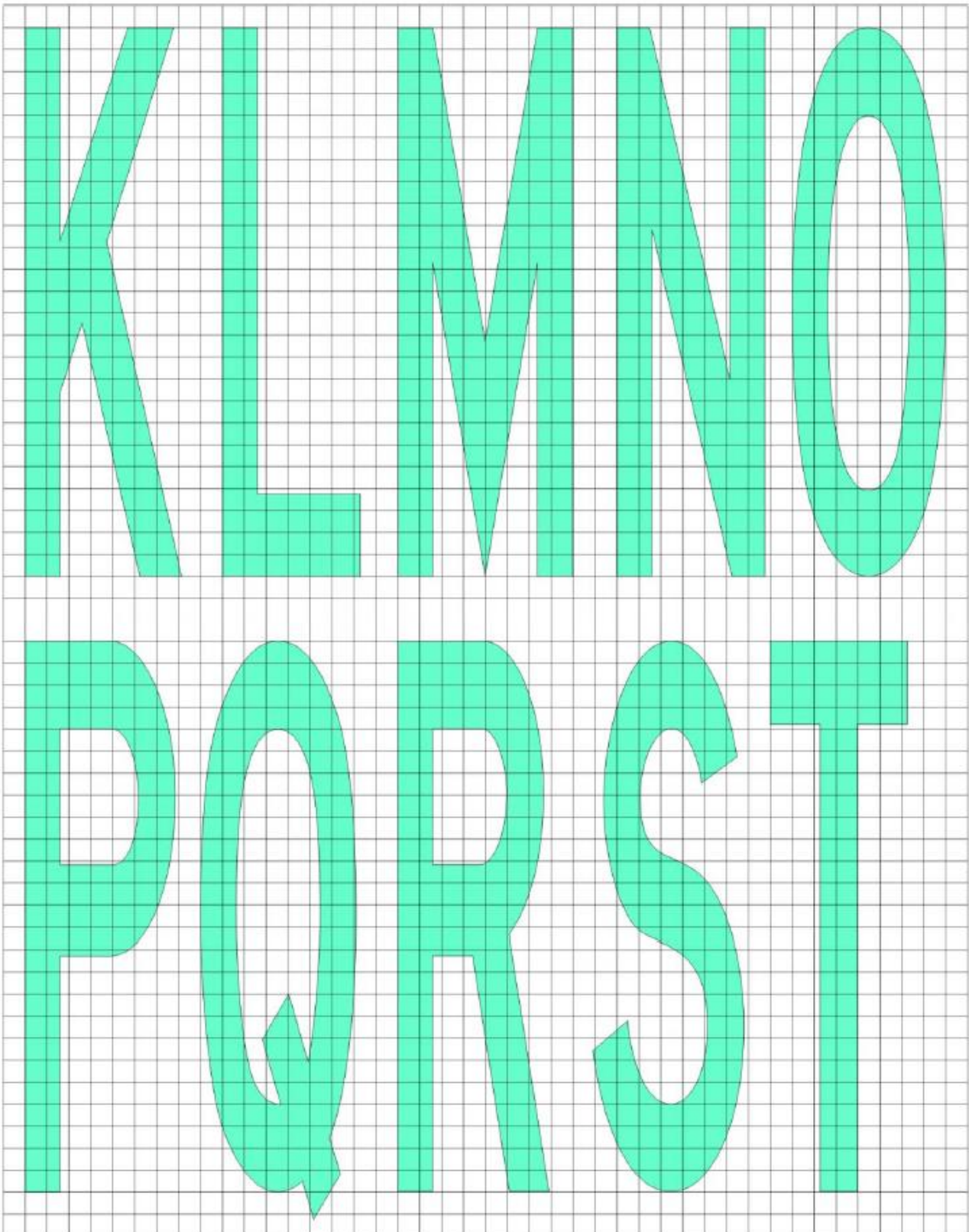
Figure L-10B. Mandatory instruction marking inscription form and proportions
