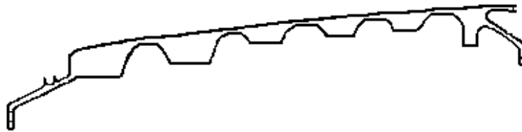
4.a - Ring Disk Drum Rotor Cross Section
