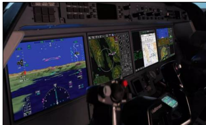
Figure 6: SVS implementation on a PFD (Source: Honeywell )
