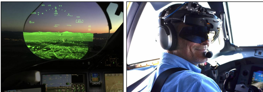
Figure 1: EFVS implementations: HUD (left), HUD equivalent wearable display (right) (Sources: Dassault Aviation and Elbit systems )
