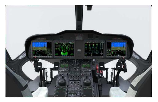
The instrument panel and inter-seat console contain all the control panels and displays governing the systems installed in the aircraft and utilised by the flight crew. The overhead console is installed above the heads of the flight crew and includes the circuit breaker panels and the rotor brake control lever.
