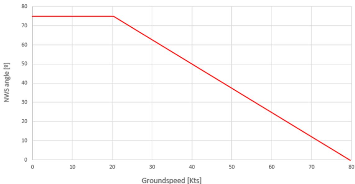
The issue identified was that a rapid speed reduction during high-energy braking could result in an equally rapid increase in the nose-wheel angle permitted by the NWS system. This rapid change can create a situation where the nose wheel turns sharply, causing the aircraft to yaw suddenly, which the pilot might not be able to counteract in time.
