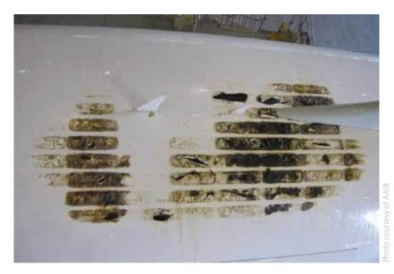
Damage to aircraft skin and fuselage resulting from an internal battery fire
