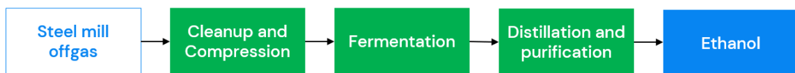
► Figure 29: Simplified block flow diagram of steel mill offgas to ethanol process
