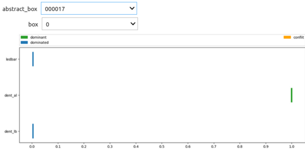
Figure 147 – Detailed view of the stability of the classification (confidence parameter) of a box using formal method. In this case the box is stable on its classification dent_al
