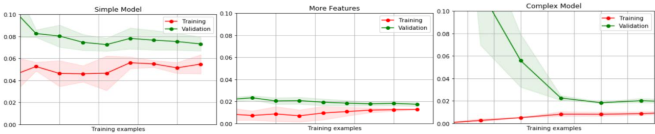
Figure 83. Learning curves 86 showing the error evolution of different models with different complexities
