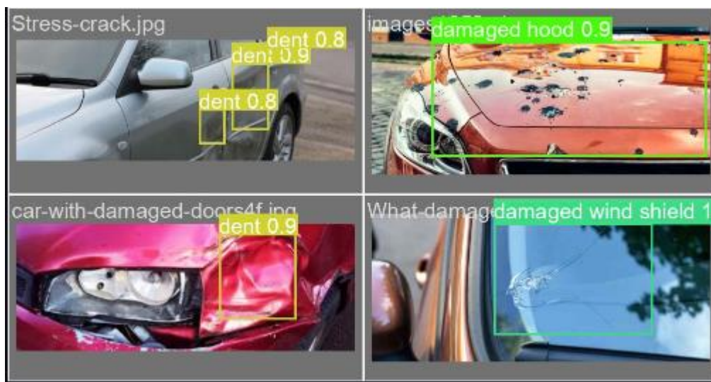
Figure 118. Example of some damages detected with the trained model showing the kind of damages present in the dataset
