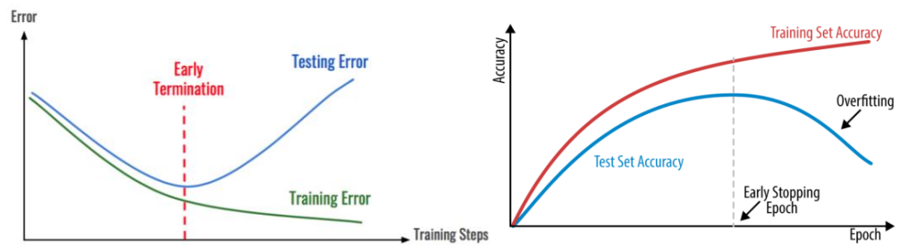
Figure 87. Illustration of the early stopping strategy based on error (left 103 ) and accuracy (right 104 ) evolution during training in test and training sets.
