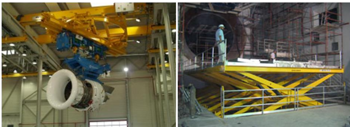
Figure 77 Left: Stock image of an aircraft engine linked to the engine carrier frame (blue) and being moved on the ceiling mounted mono-rail system (yellow). Right: Stock image of an elevating floor section beneath engine in test cell for maintenance work
