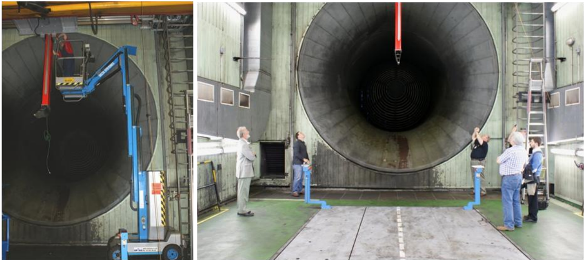
Figure 81 Photograph of new 1-D traversable probe fitted into engine test bed at SR Technics, Zurich.
