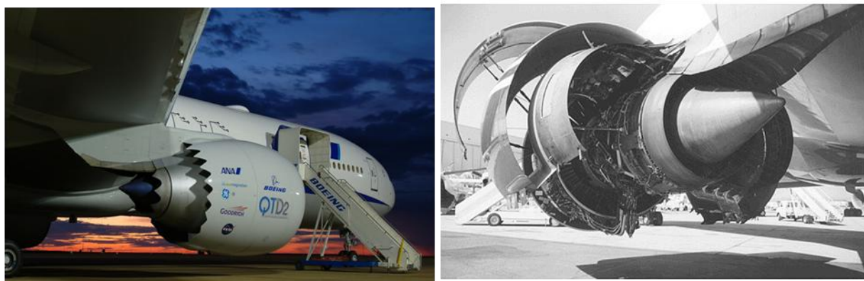
Figure 78 Left/ Right: Stock images of the tail-fairing housing that connects the engine to the aircraft wing. Note that the tail fairing must necessarily impede an area of the bypass air
