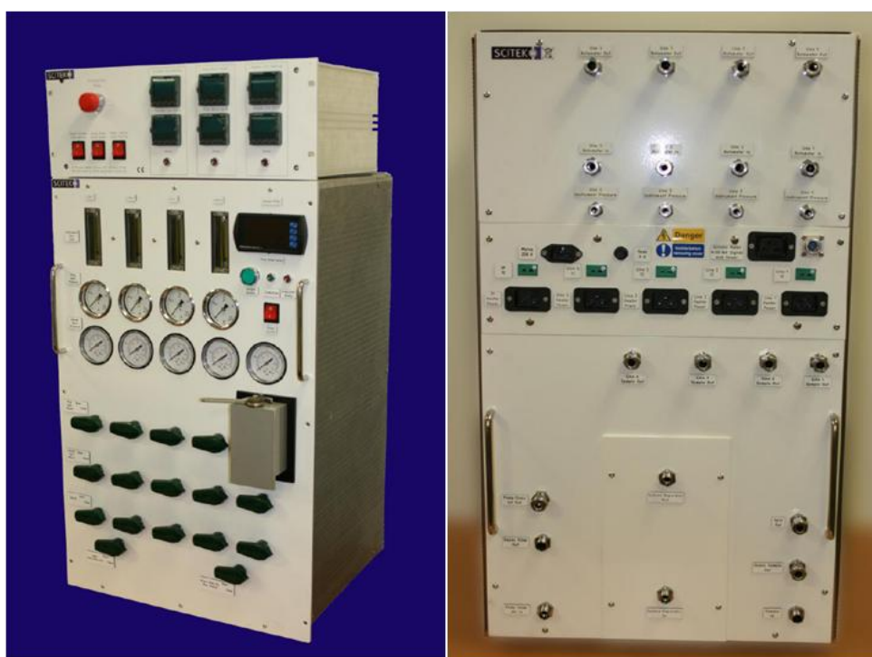
Figure 74 The front and rear panel of the console system with heater controller
