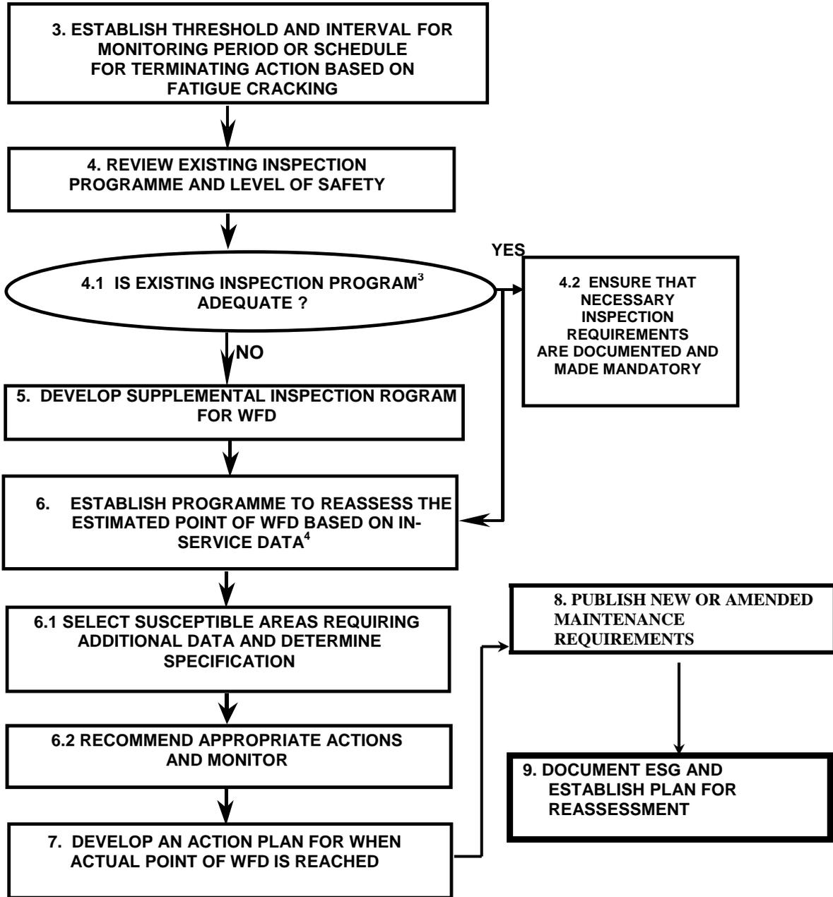
**NOTES:** 3. Inspection threshold, inspection intervals and inspection methods must be adequate to detect single or multiple cracking.
