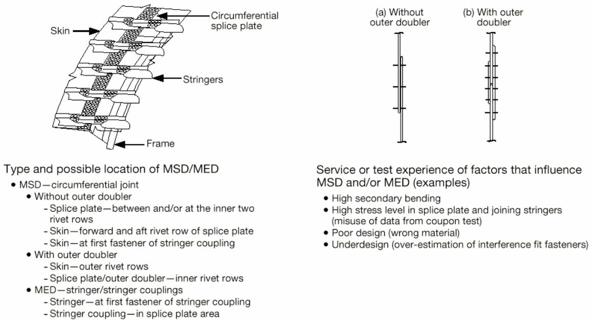
**Figure A2-2 Circumferential Joints and Stringers (MSD/MED)**
