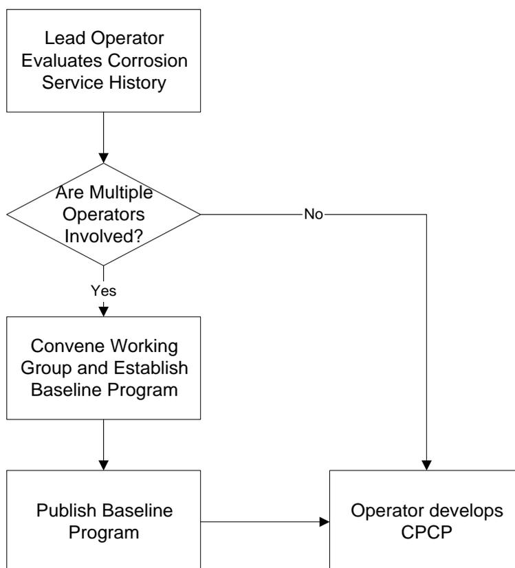
Figure 2-2. Operator Developed Baseline Program
