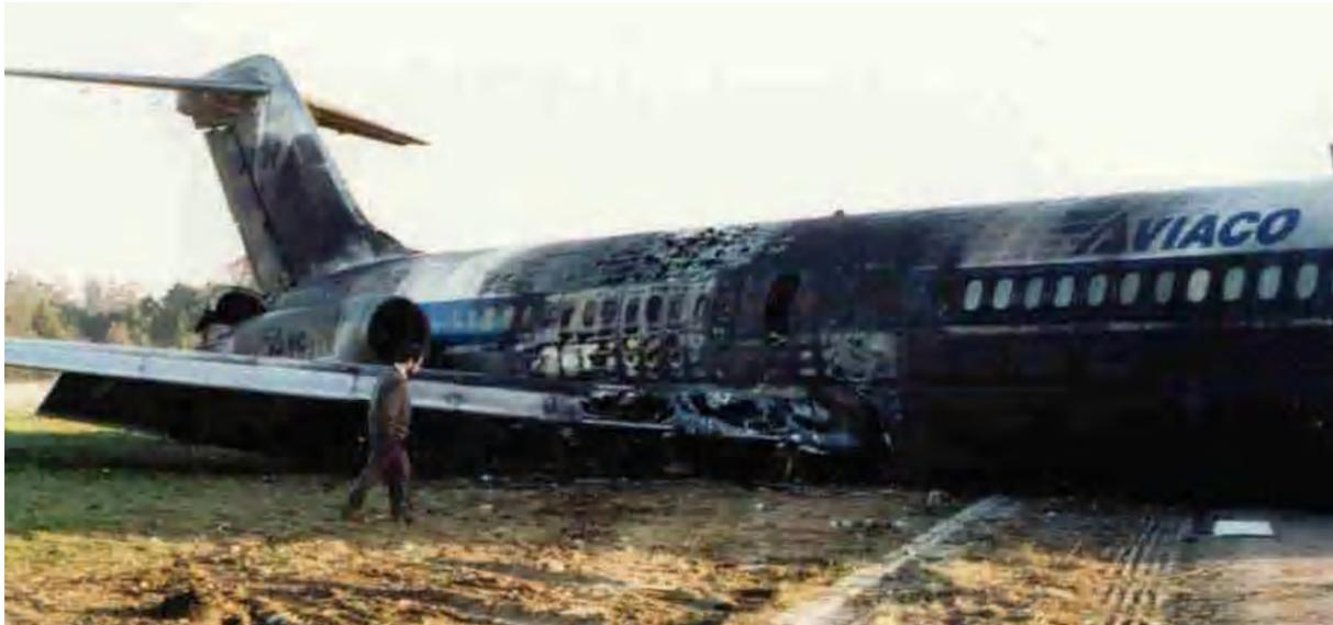
**Figure 8: Vigo DC 9-32 External Fire Damage Starboard Side**
