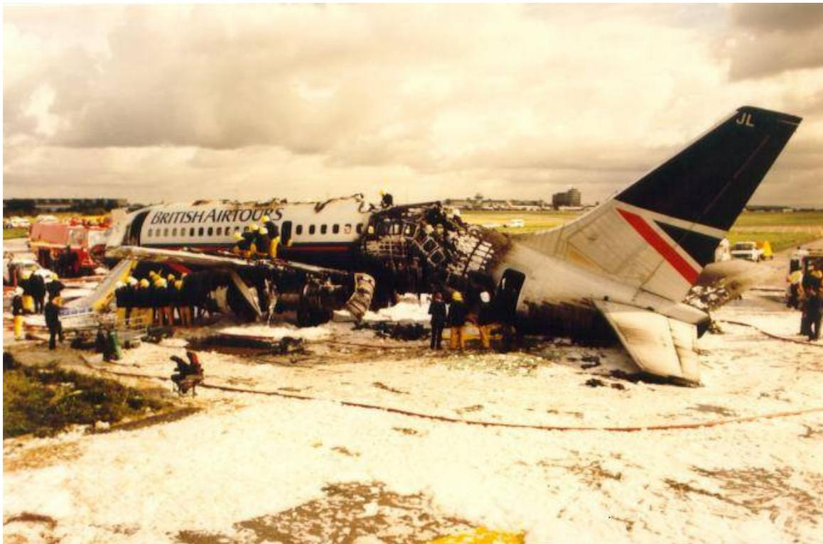
**Figure 19: Photograph of Boeing 737 Accident – Manchester England 1985 showing Structural Collapse**
