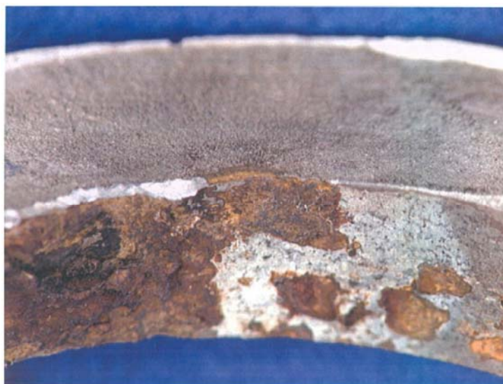
Appendix 10: Corrosion pit (tilted)
